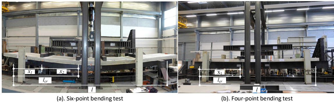
Figure 10: Photos of test setups.
