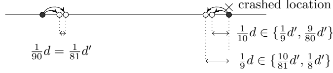
Figure 7: The possible destinations of robots after executing a move in phase B, assuming a single crashed location (on the right in this example). All the white nodes represent the possible destinations of the correct robots. We can see that regardless of where the robots end up, all the robots can detect where is the crashed location, using the ratio of the distance from an extremity to the closest robot.
