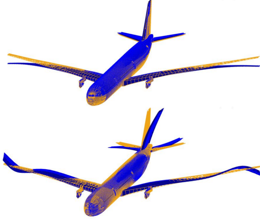
Fig. 1 First bending (up) and torsion (down) modes shapes of the XRF1-HARW
