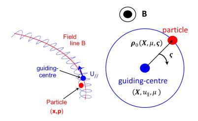
Figure 4: Decomposition of a charged particle motion into a guiding-centre position  $\mathbf{X}$  and a cyclotron motion  $\boldsymbol{\rho}$ . Strictly speaking, the cyclotron motion can be itself be separated into a periodic component, restricted here to a circular gyration  $\boldsymbol{\rho}_0$ , and a mean value, neglected here.
