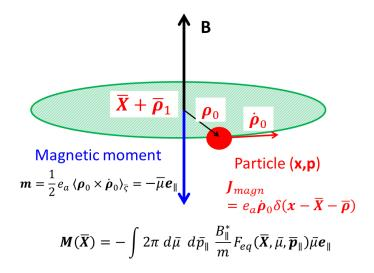
Figure 11: A particle that moves fast on a circle, a cyclotron motion, behaves as a small magnet with amplitude  $\bar{\mu}$ , with a direction opposite to the magnetic field. This process is responsible for diamagnetism in a magnetised plasma.
