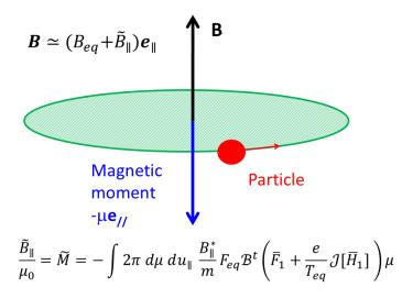
Figure 20: When submitted to a perturbed perpendicular vector potential, gyrocentres produce a perturbed magnetisation field  $\tilde{\mathbf{M}} = \tilde{M}\mathbf{e}_{\parallel}$ . In first approximation the compressional component of the magnetic field  $\tilde{B}_{\parallel}$  is proportional to the perturbed magnetisation  $\tilde{B}_{\parallel} = \mu_0 \tilde{M}$ , which yields an explicit expression of  $\tilde{B}_{\parallel}$  versus a moment of the gyrocentre distribution function.
