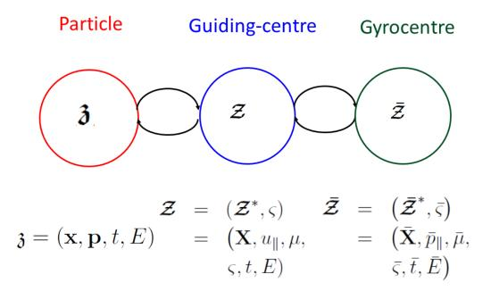
Figure 5: Sequence of transforms from particle to guiding-centres, then to gyrocentres. A complete gyrokinetic theory must provide the two corresponding changes of variables, to move back and forth from one representation to the others.
