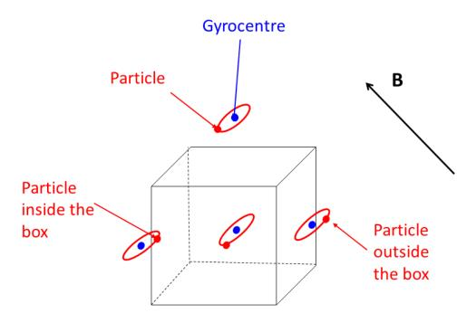
Figure 12: Calculation of the particle density knowing the distribution of gyrocentres. When counting particles in a box, some particles have their gyrocentres outside the box, while the opposite may also appear. When the plasma is inhomogeneous, this leads to differences between the densities of particles and gyrocentres. A detailed calculation leads to a particle density in accordance with Eq.(49).
