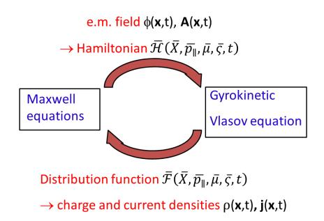
Figure 9: Schematics of a self-consistent gyrokinetic model. The electromagnetic field produces an Hamiltonian that is written in gyrocentre coordinates to solve the gyrokinetic equations. The resulting distribution function is used to compute particle charge and current densities, which are then inserted in the Maxwell equations in the physical space to produce an updated electromagnetic field.
