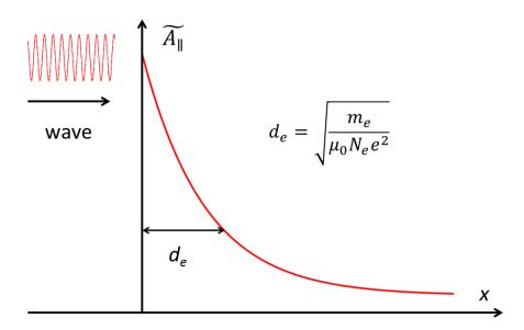
Figure 18: Illustration of the plasma skin depth effect. The amplitude  $A_{\parallel}$  of a high frequency electromagnetic wave that comes from the left decays exponentially when entering the plasma at x = 0. The decay length is the collisionless skin depth  $d_e$ .
