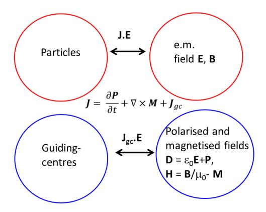
Figure 23: Particle/field energy exchange. Upper panel: particles and electromagnetic field exchange energy via the product  $\tilde{\mathbf{J}} \cdot \tilde{\mathbf{E}}$ . Lower panel: in the guiding-centre stand point, the kinetic energy is associated with guiding-centres - the polarisation and magnetisation terms enter the electromagnetic energy via the polarised and magnetisation fields.
