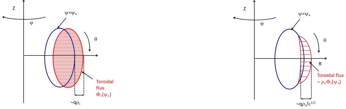
Figure 15: Poloidal cut of particle drift surfaces in a tokamak. Drift surfaces of passing particles are horizontally shifted by a distance \sim q\rho_c (left panel). The flux of the toroidal field is close to the reference magnetic flux. Trapped particles show a characteristic banana shape. The width is of the order of \sim \frac{q\rho_c}{\sqrt{\epsilon}} (right panel). Banana tips are bounce points where the parallel velocity vanish. The flux of the toroidal field is small and vanishes in the limit of small magnetic drift.
