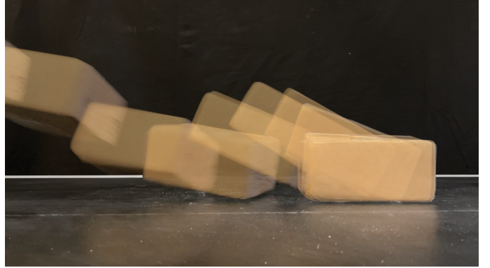
Fig. 1: Example of a tossing experiment. In a typical experiment, the box travels about 1.2 meters, impacts, and slides over the conveyor before it comes to rest. A motion capture system records the poses of the box and the conveyor at 360FPS.
