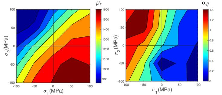
Figure 5: Experiments: biaxial stress influence on (a) initial anhysteretic relative permeability  $\mu_r$ ; (b) magnetostriction sensitivity parameter  $\alpha_{||}$  for magnetostriction along applied field.
