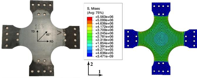
Figure 2: Cross shaped specimen and finite element calculation representing the von-mises equivalent stress ( $F_1 = F_2 = 500\text{N}$ ) - arrows (1,2) indicate the specimen frame and directions of applied forces.
