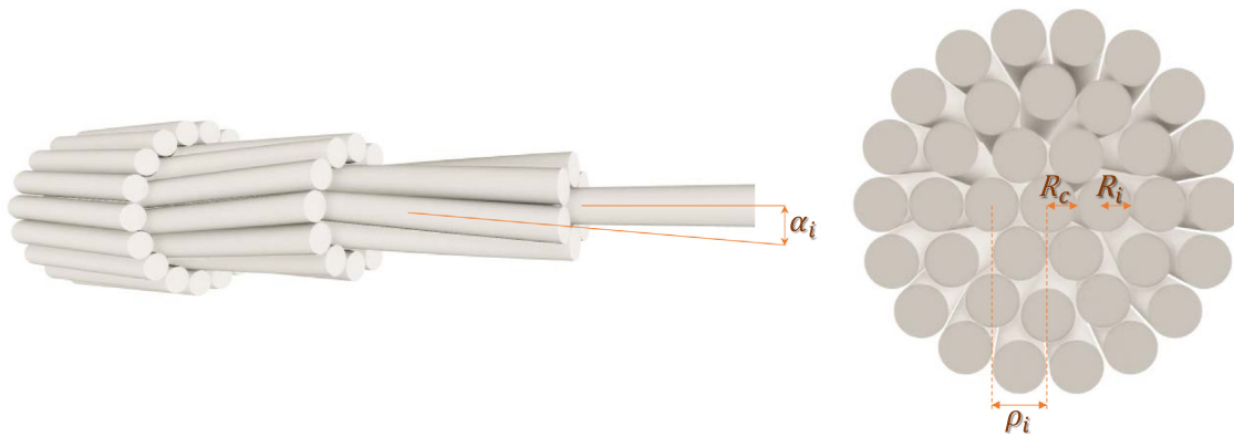
Fig. 1. The side view, internal configuration and cross section of a spiral strand.
