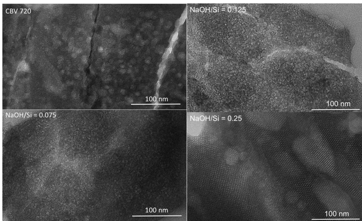
**Fig. 1.** Transmission electron microscopy images of the starting zeolite (FAU-Y, named CBV 720) and of the mesoporous FAU exhibiting mesoporosity obtained using different NaOH/Si molar ratios: NaOH/Si 0.075, 0.125, 0.25. The scale is shown on each image. The dark regions show the pore walls while the light regions show the pore voids.
