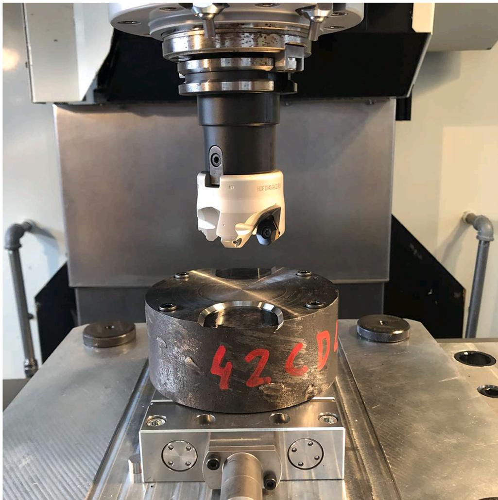
**Fig. 2.** Experimental setup for milling tests.
