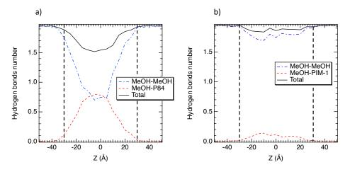
Figure 4: z-axis profile of the number of hydrogen bonds (per molecule) formed between MeOH molecules themselves and between MeOH molecules and the membrane in a) the P84 membrane and b) the PIM-1 membrane. The dashed vertical lines indicate the membrane/solvent interfaces.
