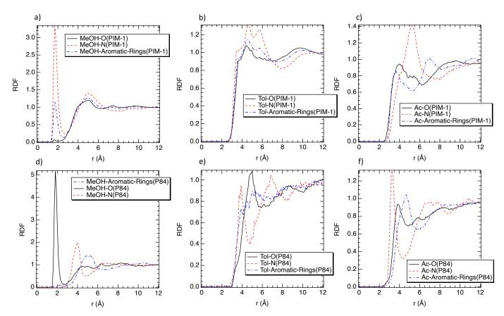
Figure 5: Radial distribution functions (RDF) between the center of mass of the solvent molecules and the oxygen atoms, nitrogen atoms and aromatic rings of the PIM-1 membrane (figures a, b and c) and the P84 membrane (figures d, e and f).
