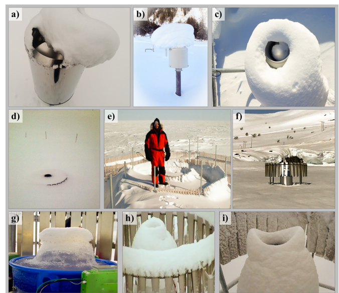
Fig. 6. Photos of common solid precipitation measurement issues, such as (a),(b),(c),(h),(i) fully or partially capped gauges; (d),(f) buried gauges; (e) shields that have accumulated drifting snow; (g) gauges with frozen bucket contents; and (h),(i) shields that have accumulated snow.
