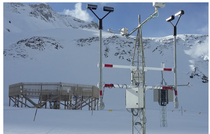
Fig. 7. Disdrometer intercomparison at the Formigal SPICE site in Spain, with the DFAR in the background.
