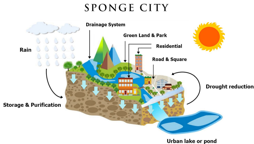
Fig. 2 Water cycle in a sponge city. By contrast with traditional urban drainage systems based on pipes and channels, initiated in Paris and other European cities during the first half of the nineteenth century (Burian and Edwards 2012), the sponge city integrates green infrastructures that allow infiltration, purification, and storage of rainwa-
