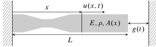
**Figure 1:** System of interest: a one-dimensional bar with non-constant cross-sectional area.
