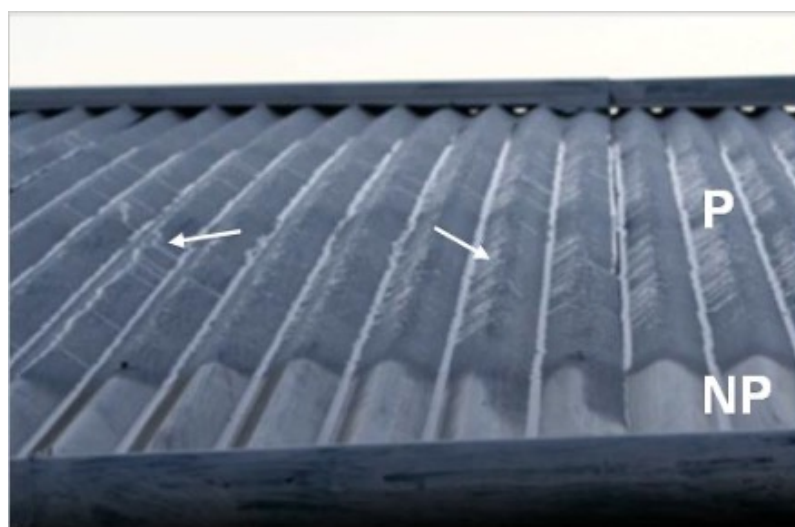
Figure 4. drops sliding on a corrugated galvanized iron roof in Combarbala, Chile, with a small angle of inclination ( \approx 15^\circ ). P: Part painted with additives (OPUR [12] ) where dew forms and drops slide on the corrugations (arrows). NP: Unpainted part where dew does not form. [Source: J.-G. Minonzio]
