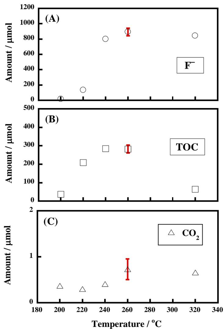
**Figure 10.** Temperature dependence of ETFE decomposition using NaOH in the presence of O<sub>2</sub>: (A) the F<sup>-</sup> amount in the reaction solution, (B) the TOC amount in the reaction solution, and (C) the CO<sub>2</sub> amount in the gas phase. The reaction conditions were the same as those described in the caption of Figure 9 (NaOH), except that O<sub>2</sub> was used instead of Ar. Error bars at 260 °C were obtained from two replicate experiments under the same reaction conditions.
