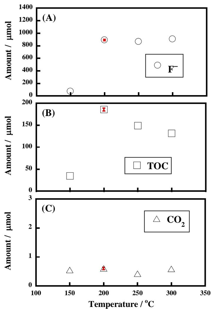
**Figure 5.** Temperature dependence of PVDF decomposition in the presence of O<sub>2</sub>: (A) the F<sup>-</sup> amount in the reaction solution, (B) the TOC amount in the reaction solution, and (C) the CO<sub>2</sub> amount in the gas phase. The reaction conditions were the same as those described in the caption of Figure 3, except that O<sub>2</sub> was used instead of Ar. Error bars at 200 °C were obtained from two replicate experiments under the same reaction conditions.
