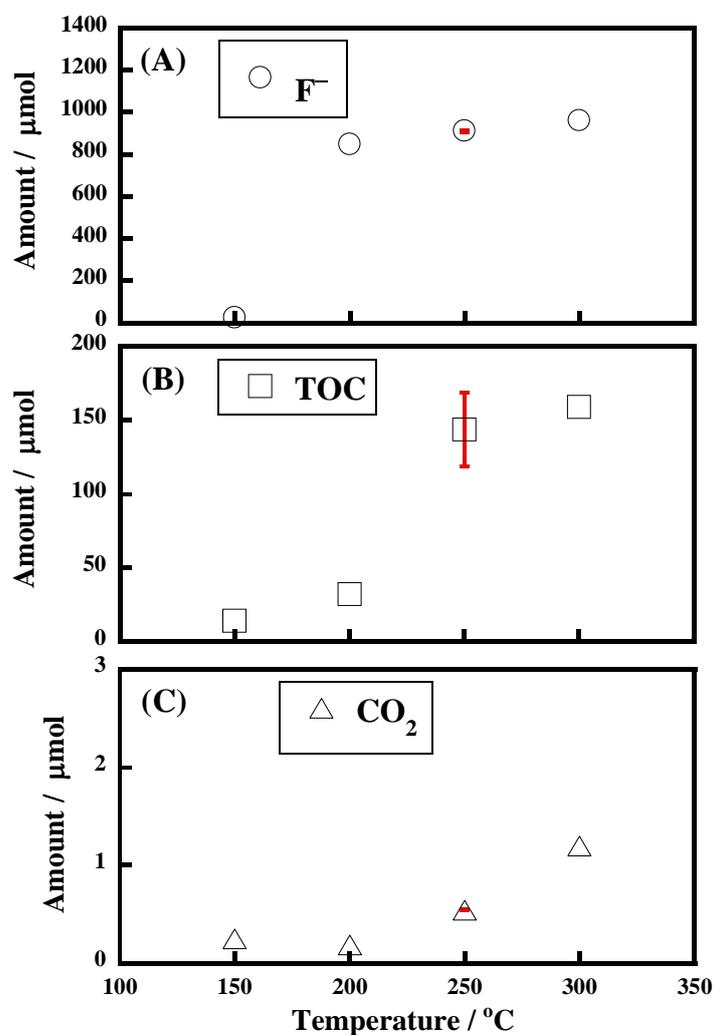
**Figure 3.** Effect of temperature on (A) the  $F^-$  amount in the reaction solution, (B) the TOC amount in the reaction solution, and (C) the  $CO_2$  amount in the gas phase. PVDF (30 mg) was reacted in the presence of 1.0 M of [KOH] in superheated water under Ar for 6 h. Error bars at 250 °C were obtained from two replicate experiments under the same reaction conditions.
