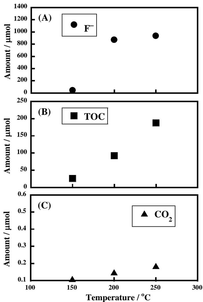
**Figure 7.** Effect of temperature on (A) the  $F^-$  amount in the reaction solution, (B) the TOC amount in the reaction solution, and (C) the  $CO_2$  amount in the gas phase. Poly(VDF-*co*-HFP) copolymer (30 mg, fluorine amount as atoms; 938 μmol; carbon content as atoms, 902 μmol) was reacted in the presence of 1.0 M of [KOH] in superheated water under Ar for 6 h.
