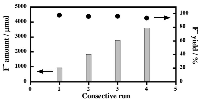
**Figure 6.** F<sup>-</sup> amount and F<sup>-</sup> yield after consecutive runs for PVDF decomposition. PVDF (30 mg) was reacted with 1.0 M of [KOH] in superheated water at 250 °C under Ar for 6 h. After the reaction, the autoclave was cooled to room temperature, and new PVDF (30 mg) was charged to the resulting reaction mixture, purged with Ar, then the mixture was further heated at 250 °C for 6 h.
