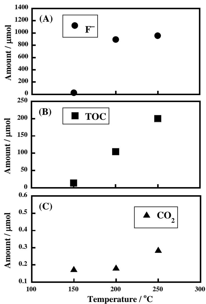
**Figure 8.** Temperature dependence of poly(VDF-*co*-HPF) copolymer decomposition in the presence of O<sub>2</sub>: (A) the F<sup>-</sup> amount in the reaction solution, (B) the TOC amount in the reaction solution, and (C) the CO<sub>2</sub> amount in the gas phase. The reaction conditions were the same as those described in the caption of Figure 7, except that O<sub>2</sub> was used instead of Ar.
