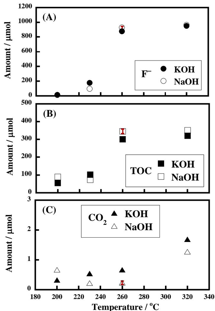
**Figure 9.** ETFE reactions using KOH or NaOH in a bigger autoclave (96 mL): Effect of temperature on (A) the  $F^-$  amount in the reaction solution, (B) the TOC amount in the reaction solution, and (C) the  $CO_2$  amount in the gas phase. ETFE (30 mg) was reacted in the presence of 1.0 M of [KOH] or [NaOH] in superheated water under Ar for 6 h. Error bars for the reaction using NaOH at 260°C were obtained from two replicate experiments under the same reaction conditions.
