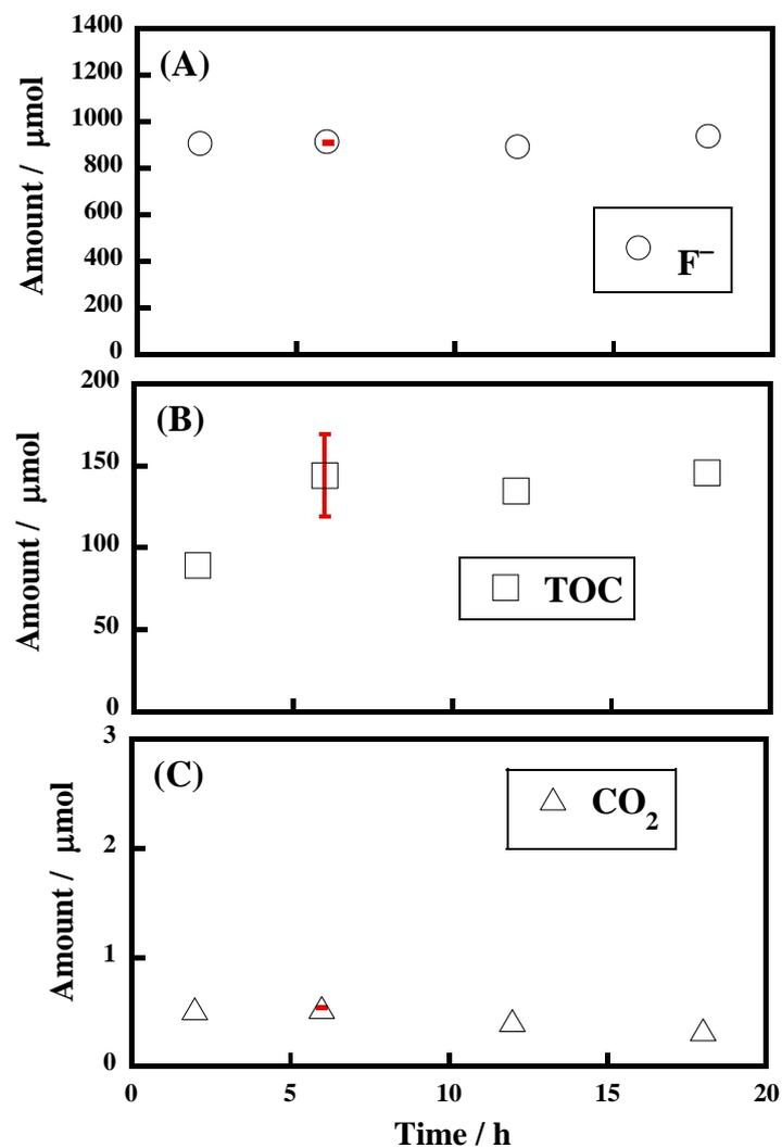
**Figure 4.** Effect of reaction time on (A) the  $\text{F}^-$  amount in the reaction solution, (B) the TOC amount in the reaction solution, and (C) the  $\text{CO}_2$  amount in the gas phase. PVDF (30 mg) was reacted in the presence of 1.0 M of [KOH] under Ar in superheated water at 250 °C. Error bars at 6 h were obtained from two replicate experiments under the same reaction conditions.
