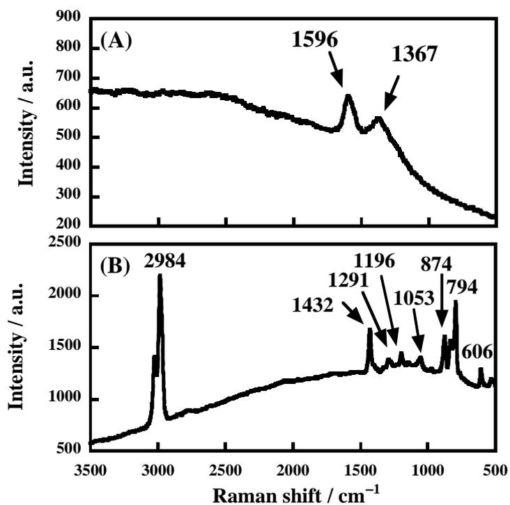
**Figure 2.** Raman spectra of (A) the solid residue formed from a reaction of PVDF in superheated water with 1.0 M of [KOH] under Ar and (B) PVDF before the treatment. For (A), the treatment was performed at 250 °C for 6 h.
