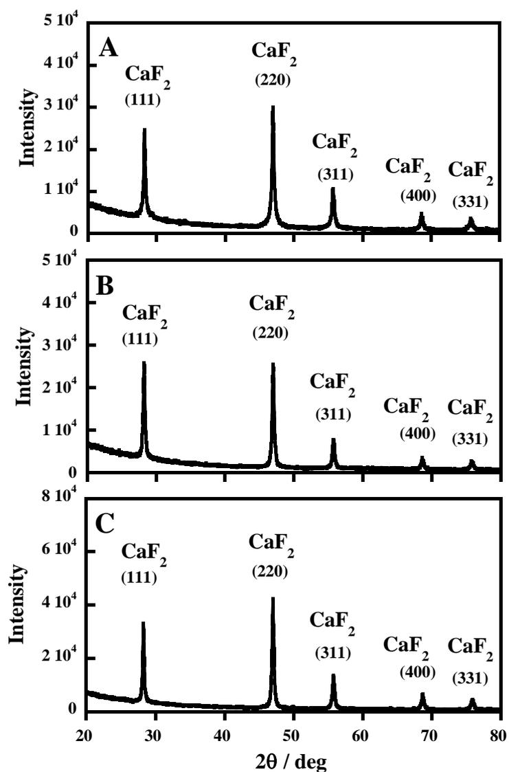
**Figure 11.** XRD patterns of the artificial fluorspar obtained from (A) PVDF, (B) poly(VDF-*co*-HFP) copolymer, and (C) ETFE. Ca(OH)<sub>2</sub> was added to the reaction solution from superheated water treatment, and the formed precipitate was washed with aqueous HCl and pure water, and dried.
