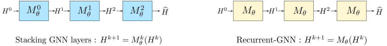
Figure 6. Comparison between a usual GNN architecture (left) where different Message Passing layers M_\theta^i are stacked (i.e. the weights are different for all layers) and a Recurrent-GNN structure where the solution \hat{H} is computed iterating on the same Message Passing layer.
