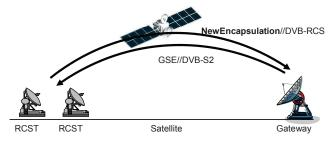
Figure 3: Forward and return link encapsulation
