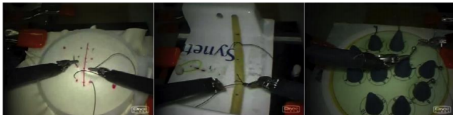
Fig. 1 Sample frames from the three tasks in the JIGSAWS dataset, from left to right: Suturing frame, Knot-Tying frame, Needle-Passing frame.
