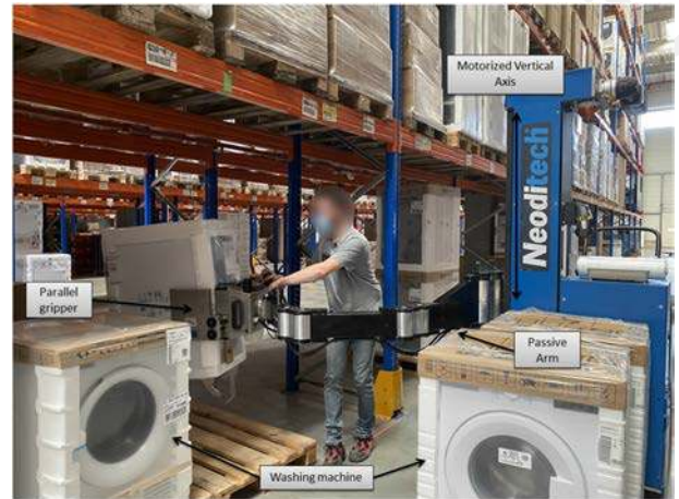
Fig. 1. Example from washing-machine pick and place manipulation with a Neoditech Scara parts arm.
