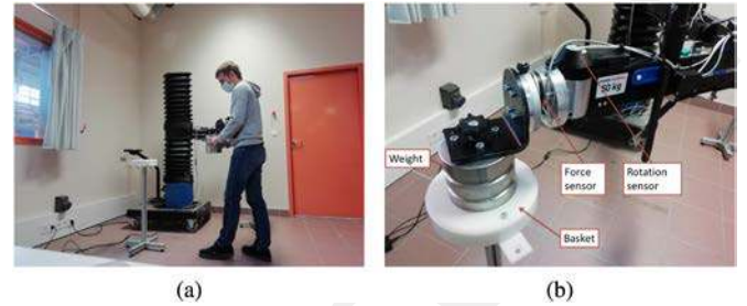
Fig. 4. (a) User performing the experiment. (b) Sensor setup, weight manipulated.
