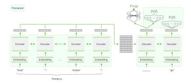
Figure 8: GFlan-T5: We use the Flan-T5 architecture and add a value head. We initialize the agent with the pretrained weights (framed in green in the diagram) including its language modeling heads to compute action probabilities. The weights of the value head are initialized randomly. GFlan-T5 stands for: grounded Flan-T5.
