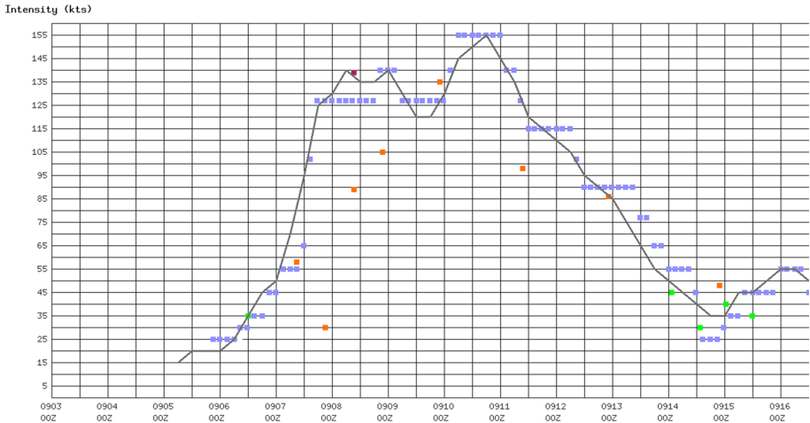
Fig. 21 Intensity (kt) versus Time (month and day) estimated from the Dvorak method (light blue squares), ASCAT (green squares), SMAP (orange squares), Sentinel-1 SAR (purple square), along with Joint Typhoon Warning Center intensity (black line) for Chanthu (19th TC of the 2021 western North Pacific season)
