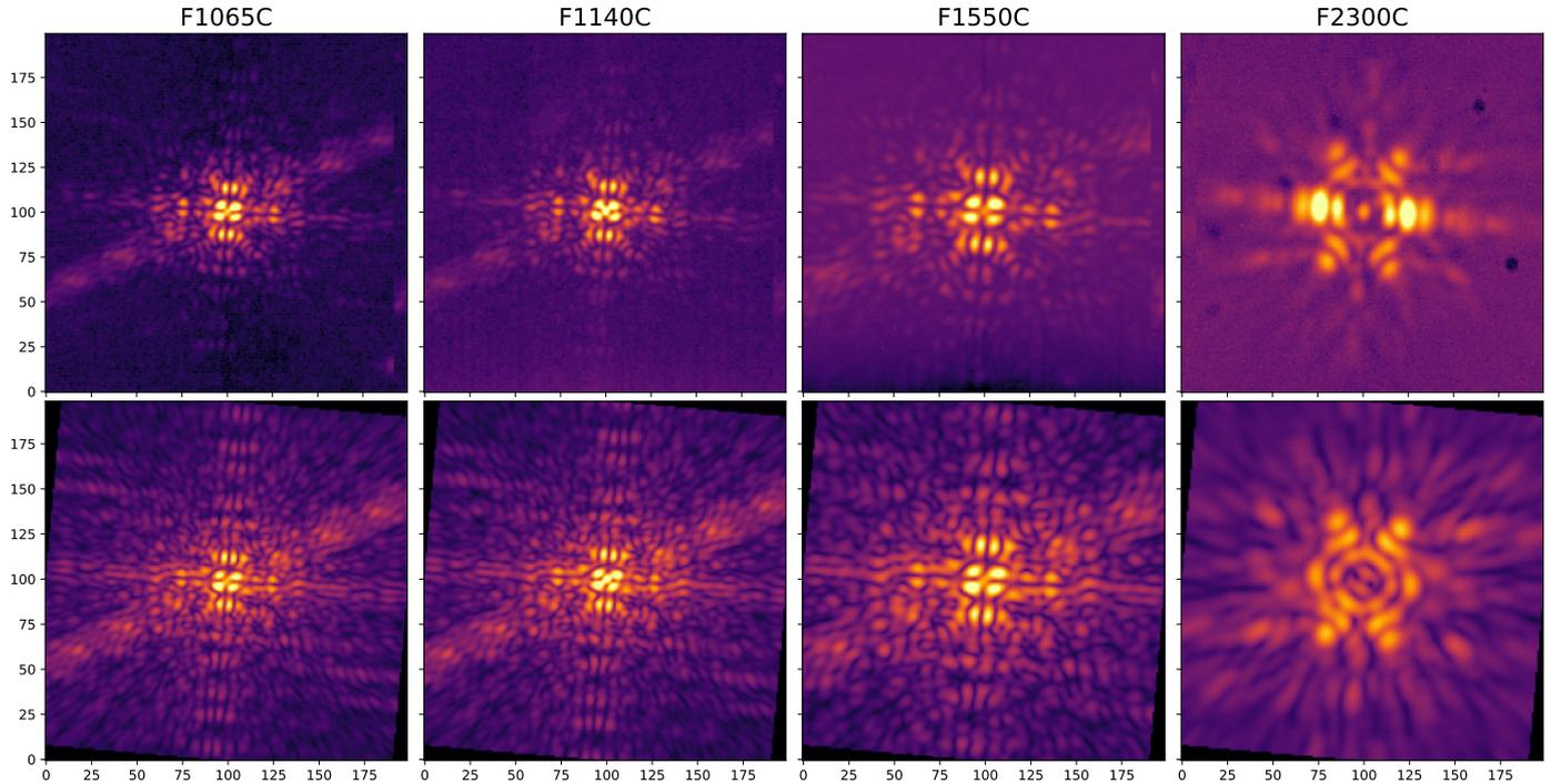
**Fig. 3.** Observed (*top*) versus simulated (*bottom*) coronagraphic images (on-axis) in the four coronagraphic filters. The pixel scale is 110 mas. Dark spots in the F2300C image correspond to background stars recorded during the background observation. Simulated data use the nominal scenario (see Table 3). The intensity scale is not linear.
