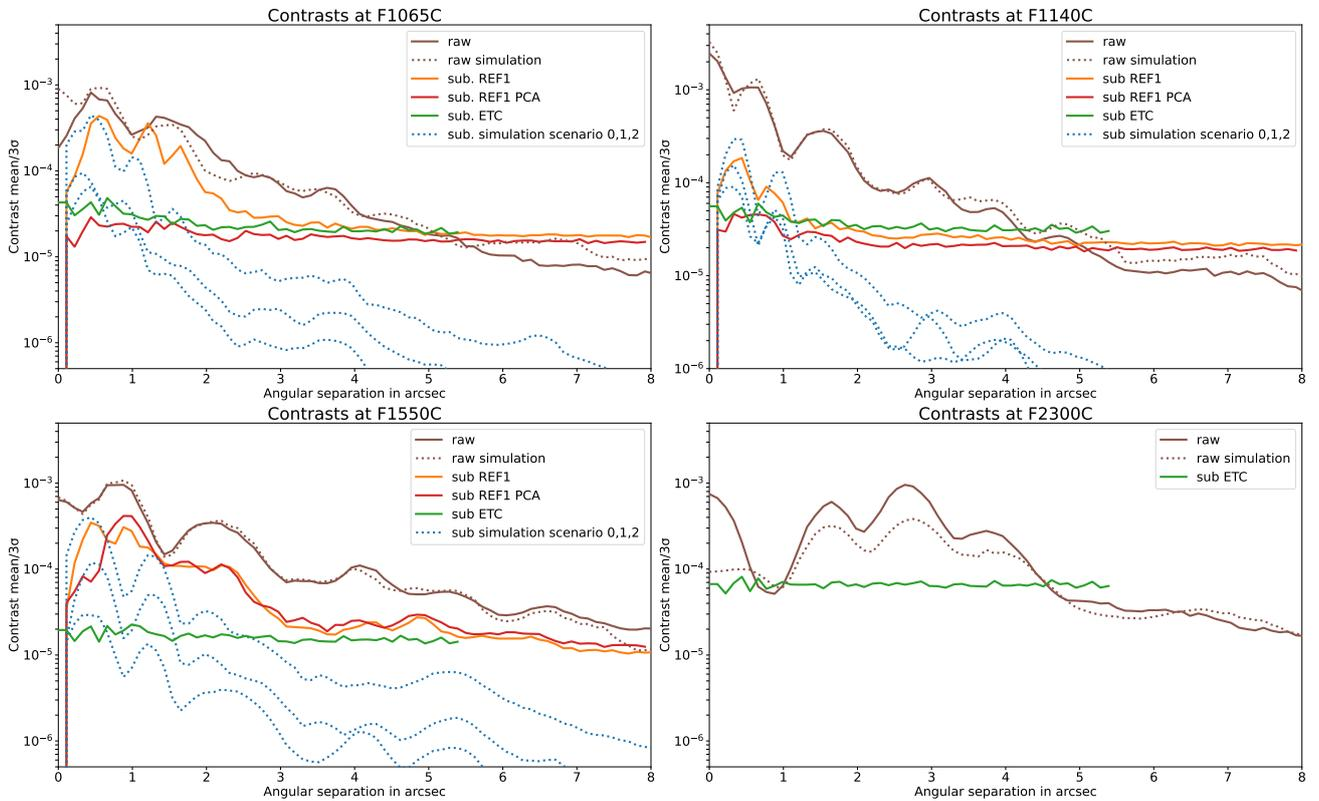
**Fig. 5.** Measured raw and  $3\sigma$  reference-star-subtracted contrasts for all MIRI coronagraphic filters as compared to the simulations and to the ETC prediction. Subtracted contrasts are shown for the one-to-one and PCA algorithms. Reference stars were not observed at F2300C.
