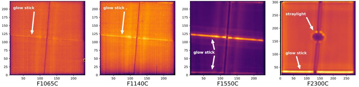
**Fig. 1.** Images of the background obtained in the coronagraphic subarrays showing the “glow sticks” visible at the horizontal transitions of the 4QPMs and around the disk of the Lyot mask, as well as at the edges of the coronagraphs’ support structure. The intensity scale is linear and is adapted for each image for visualization purposes.
