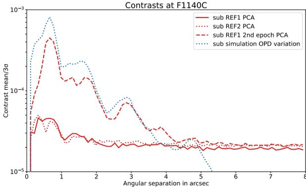
**Fig. 6.** Measured  $3\sigma$  reference-star-subtracted contrasts with PCA in the F1140C filter for the single-epoch and two-epoch cases, and compared to the simulation that takes the wavefront error maps (OPD) into account before and after re-phasing of the primary mirror segments.
