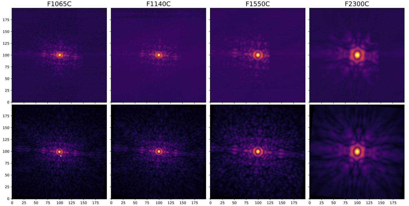
**Fig. 2.** Observed (*top*) versus simulated (*bottom*) PSFs (off-axis) in the four coronagraphic filters. The pixel scale is 110 mas. Some PSFs are cropped by the edges of the coronagraph’s mechanical support. Simulated data use the nominal scenario (see Table 3). The intensity scale is not linear.
