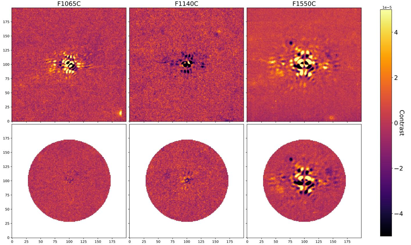
**Fig. 4.** One-to-one (*top*) versus PCA (*bottom*) subtraction of coronagraphic images (TARG and REF1) in the three 4QPM filters. Several background sources (either positive or negative) are observed around the target and reference stars. The pixel scale is 110 mas.
