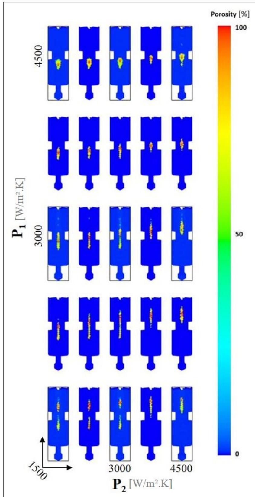
Figure 15: Our solution prediction and simulated shrinkage porosity
