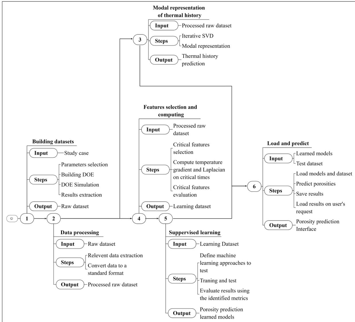
Figure 1: Flowchart of the developed porosity prediction solution
