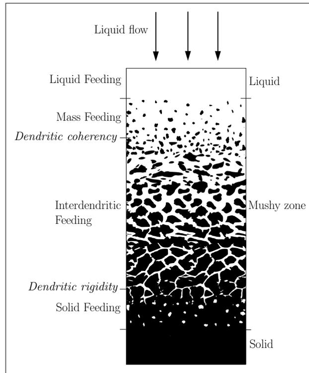
Figure 6: Different feeding mechanisms during casting process
