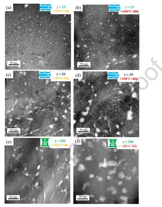
Figure 9 : STEM-HAADF images of HPS deformed alloy:  $\gamma \approx 15(a, b)$  and  $\gamma \approx 20$  (c, d) and of HTP deformed alloy (e, f) annealed 70h at 70°C (a, c, e) and 48h at 100°C (b, d, f).
