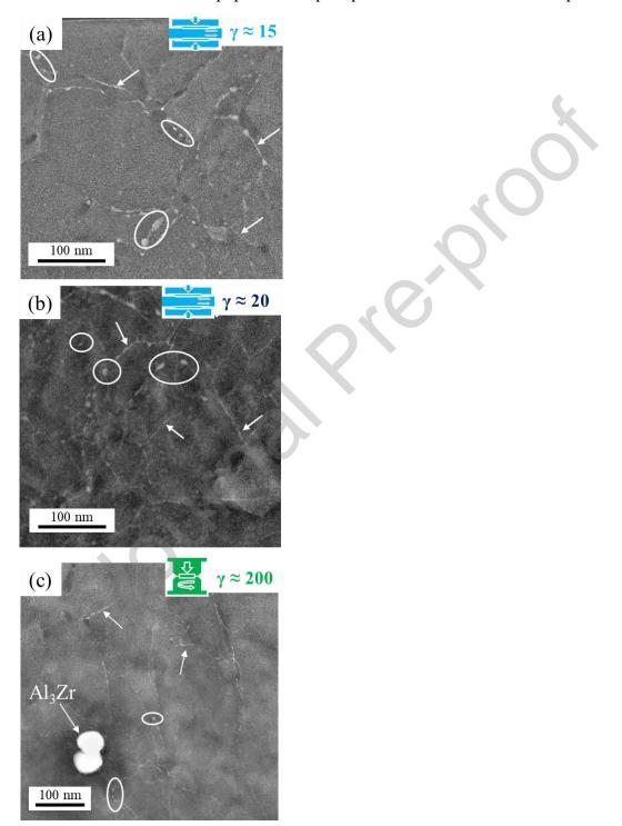
Figure 4: STEM HAADF images of as deformed alloys: HPS  $\gamma \approx 15$  (a), HPS  $\gamma \approx 20$  (b), HPT  $\gamma \approx 200$  (c).
