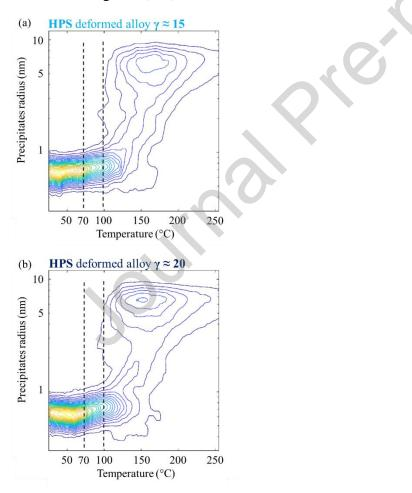
Figure 6: Precipitates size distribution estimated from SAXS data fitting during an in situ heating at 5°C/min from 20 to 250°C on HPS deformed alloy: (a)  $\gamma \approx 15$  and (b)  $\gamma \approx 20$ .
