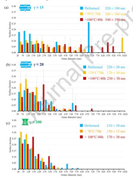
Figure 11 : Grain size distributions of HPS (a, b) and HPT (c from [5]) deformed materials before (blue) and after annealing at 70°C/70h (yellow) and 100°C/48h (red)
