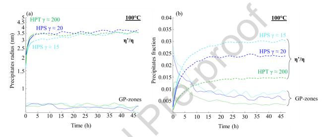
Figure 8 : Precipitate size (a) and volume fraction evolution (b) estimated from SAXS data fitting during in situ heating at  $100^{\circ}$ C on HPS (blue) and HPT (green) deformed alloys. Thin lines correspond to GPzones and thicker lines to  $\eta'/\eta$  evolutions. Dashed lines correspond to the uncertainty of the evolutions due to the SAXS detection limit.
