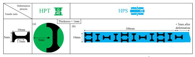
Figure 1:Schematic representation of the position of dog bone sampling on (a) HPT sample and (b) HPS sample.
