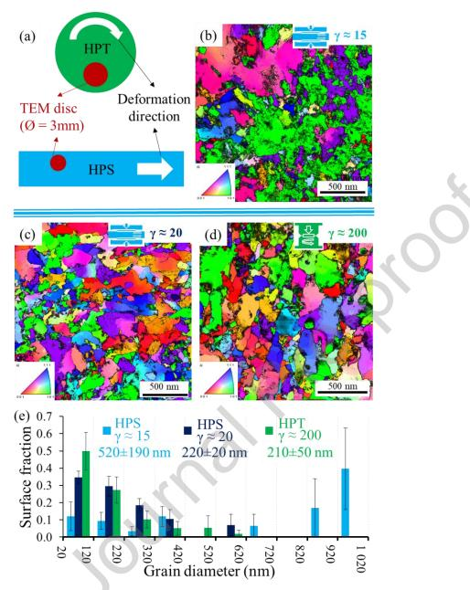
Figure 2: Schematic representation of TEM sample location for HPT and HPS samples (a). Orientation map of as deformed alloys HPS  $\gamma \approx 15(b)$ , HPS  $\gamma \approx 20(c)$  and HPT  $\gamma \approx 200(d)$ . Grain size distributions of the as deformed alloys (e).
