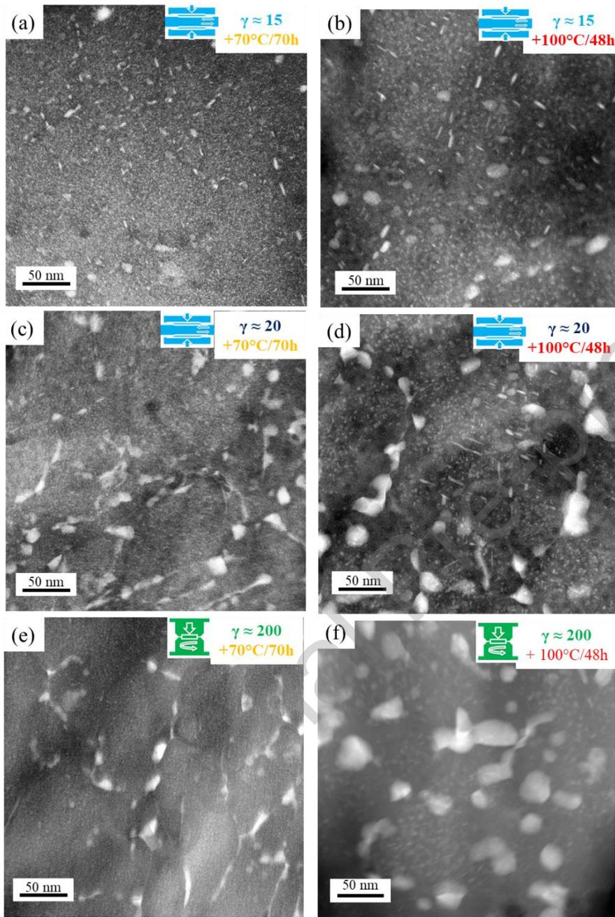
Figure 9 : STEM-HAADF images of HPS deformed alloy:  $\gamma \approx 15$  (a, b) and  $\gamma \approx 20$  (c, d) and of HTP deformed alloy (e, f) annealed 70h at 70°C (a, c, e) and 48h at 100°C (b, d, f).
