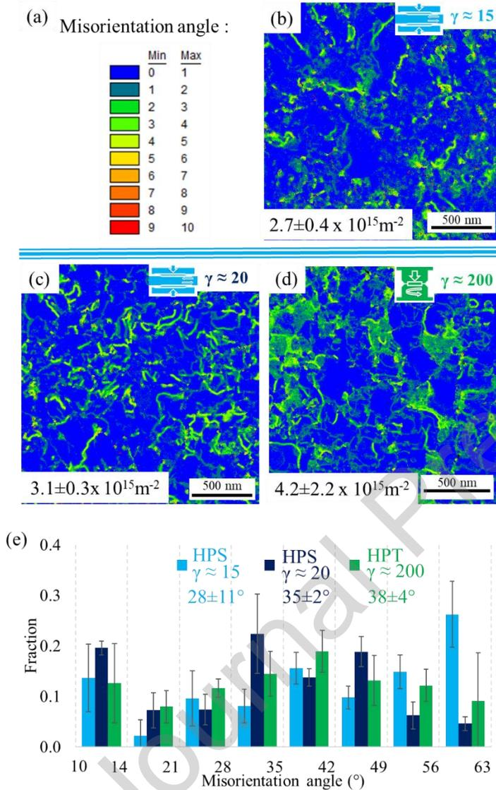
Figure 3: KAM maps (a) for as deformed sample by HPS  $\gamma \approx 15$  (b), HPS  $\gamma \approx 20$  (c) and HPT  $\gamma \approx 200$  (d). Misorientation angle distribution for HPT and HPS deformed alloys (e).
