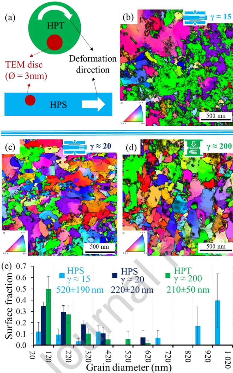
Figure 2: Schematic representation of TEM sample location for HPT and HPS samples (a). Orientation map of as deformed alloys HPS  $\gamma \approx 15$  (b), HPS  $\gamma \approx 20$  (c) and HPT  $\gamma \approx 200$  (d). Grain size distributions of the as deformed alloys (e).
