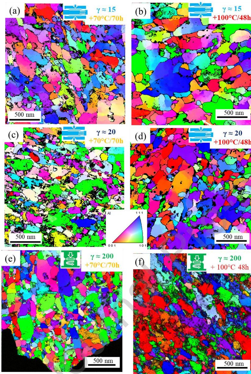
Figure 10 : TEM orientation maps of HPS deformed alloy:  $\gamma \approx 15$  (a, b) and  $\gamma \approx 20$  (c, d) and of HTP deformed alloy (e, f) annealed 70h at 70°C (a, c, e) and 48h at 100°C (b, d, f).
