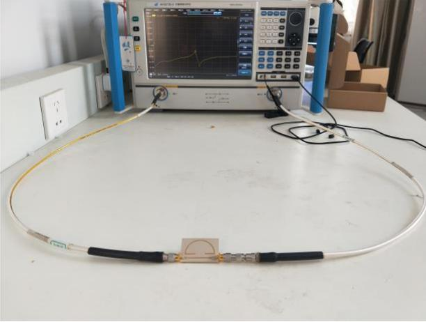
Fig. 11. Configuration of the crab-shape prototype experimental setup.
