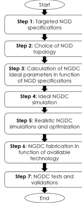
Fig. 3. Workflow of NGDC design and test method.
