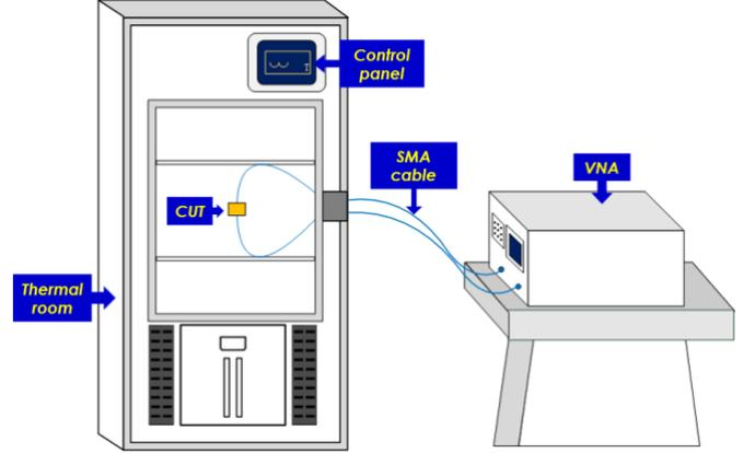
Fig. 3. Illustrative diagram of NGD electrothermal test.
