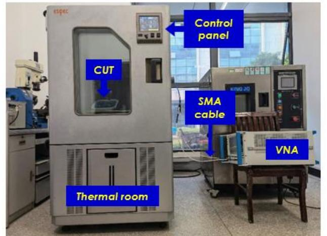
Fig. 4. Photo of the considered electrothermal experimental setup.
