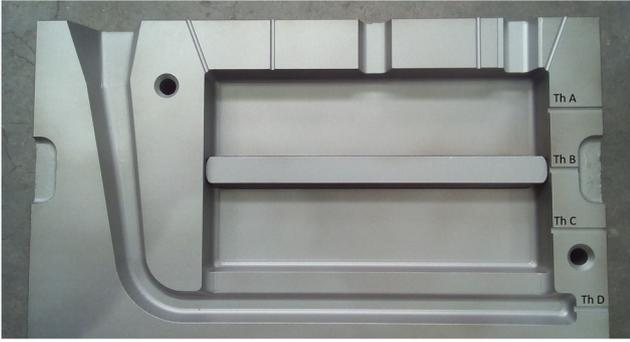
Fig. 10 The thermocouples location in the mould
