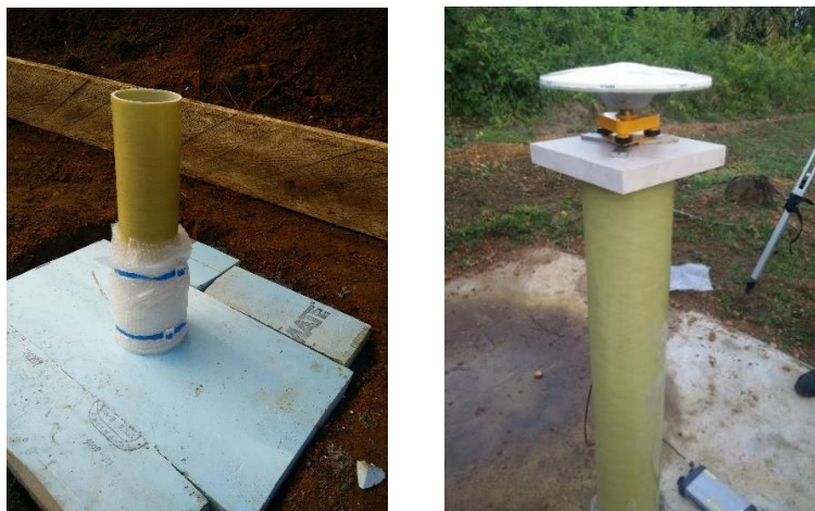
Figure 5: Creation of the vector magnetometer pillar on the left and absolute measurement pillar with a GPS to locate the place on a marble support on the right.
