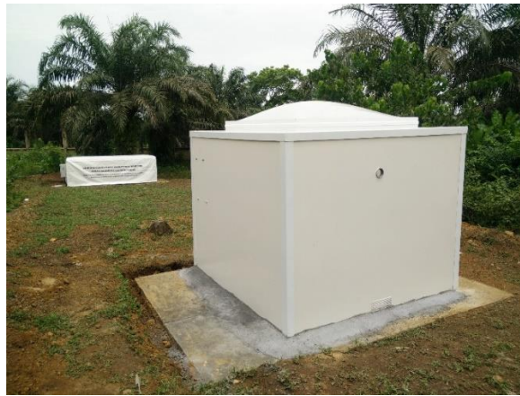
Figure 8: On the first plan, the absolute measurement pavilion and in the background, the fibreglass container housing the sensors.
