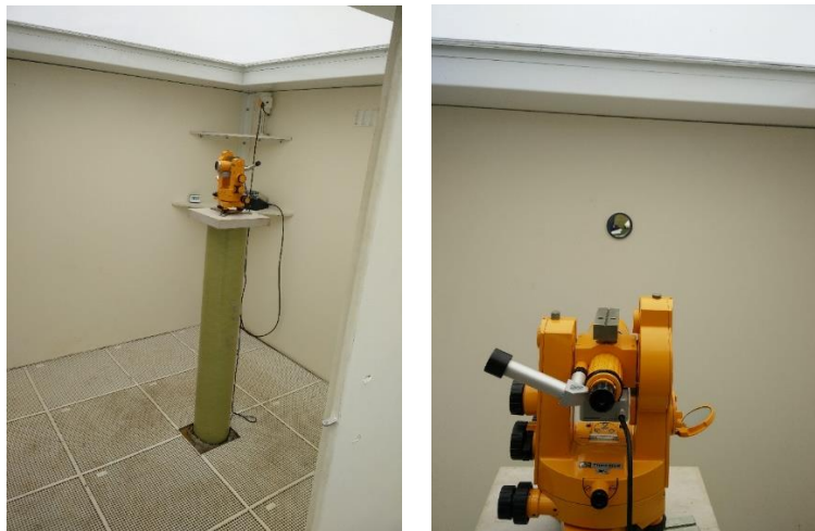
Figure 7: Inside the absolute measurement pavilion. On the left picture, the theodolite is resting on the absolute measurement pillar. On the right picture is seen the hole to aim the azimuth mark.
