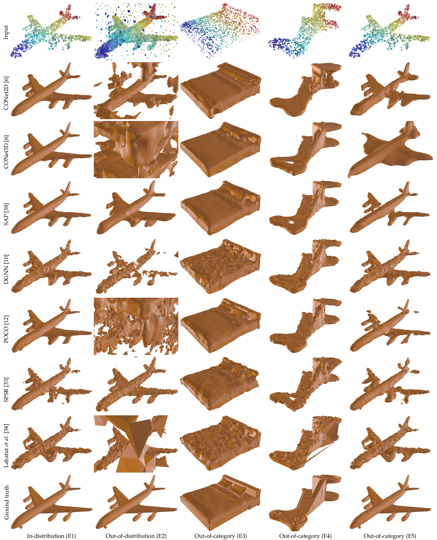
Figure 5: Learning-based reconstructions (E1 to E5): DGNN [10], SAP [38] and SPSR [33] provide visually the best reconstructions, without prevalent defects.
