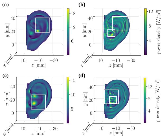
Fig. 4. Parametric surfaces for the assessment of  $S_{ab}$ . The top and bottom row correspond to polarization 1 and 2, respectively. In (a) and (c), the square averaging area of 4 cm<sup>2</sup> resulting in the maximal  $S_{ab,2}$  at 26 GHz is shown, while (b) and (d) depict the square averaging area of 4 and 1 cm<sup>2</sup> resulting in two distinct maximal  $S_{ab,2}$  at 60 GHz.
