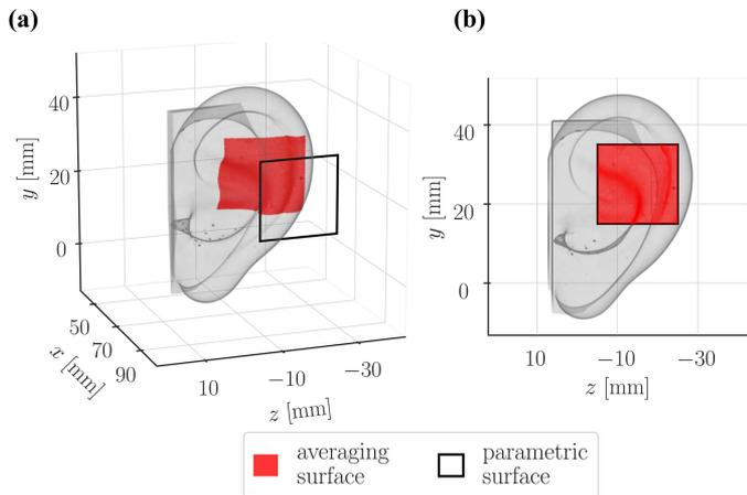
Fig. 2. Conformal surface and its corresponding 2-D parametric projection of 4 cm<sup>2</sup> area: (a) 3-D view, (b) the plane-wave incidence point of view.
