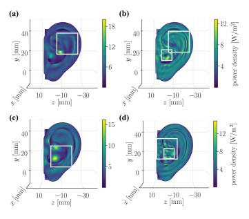
Fig. 4. Parametric surfaces for the assessment of  $S_{\rm ab}$ . The top and bottom row correspond to polarization 1 and 2, respectively. In (a) and (c), the square averaging area of 4 cm<sup>2</sup> resulting in the maximal  $S_{\rm ab,\,2}$  at 26 GHz is shown, while (b) and (d) depict the square averaging area of 4 and 1 cm<sup>2</sup> resulting in two distinct maximal  $S_{\rm ab,\,2}$  at 60 GHz.
