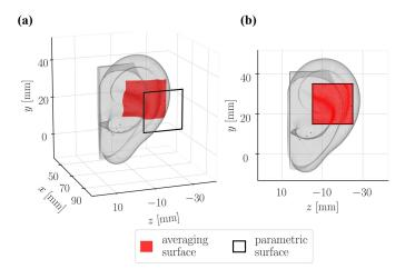
Fig. 2. Conformal surface and its corresponding 2-D parametric projection of 4 cm<sup>2</sup> area: (a) 3-D view, (b) the plane-wave incidence point of view.
