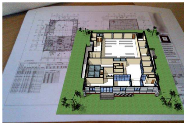
316 317 Figure 3: (left) VR tethered HMD used for measuring space between model elements [2], (right) superimposed 3D 318 view off the 2D QR-code enabled drawing using AR mobile handheld [71].
