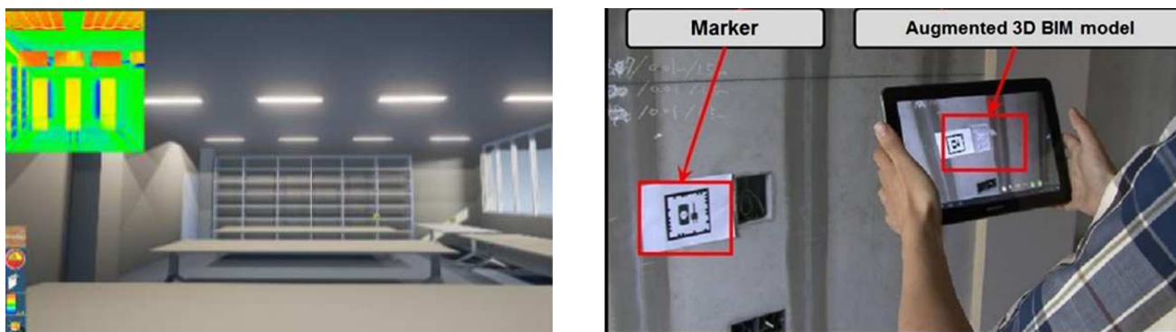
353 Figure 4: (left) Lighting simulation at daytime using VR standalone [74], (right) AR mobile handheld used on AR site- 354 experiment for quality control [78]. 355
