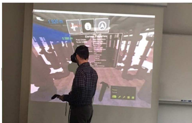
316 317 Figure 3: (left) VR tethered HMD used for measuring space between model elements [2], (right) superimposed 3D 318 view off the 2D QR-code enabled drawing using AR mobile handheld [71].
