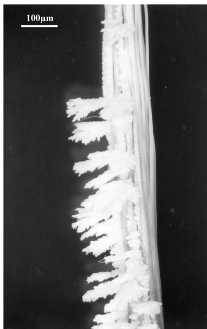
Fig. 7 Deposit processed with homogeneous nucleation ( T > 1300^{\circ}\text{C} )
