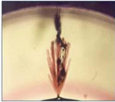
Typical water treeing in MV XLPE cables manufactured from 1978 - 1986.
