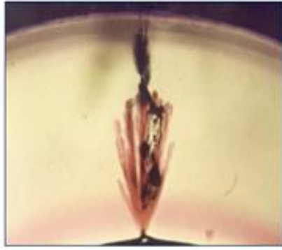
Typical water treeing in MV XLPE cables manufactured from 1978 - 1986.
