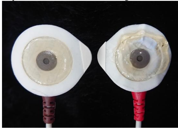
Fig. 22. Initial (left) and final (right) state of wet electrodes used during pressure variation tests.
