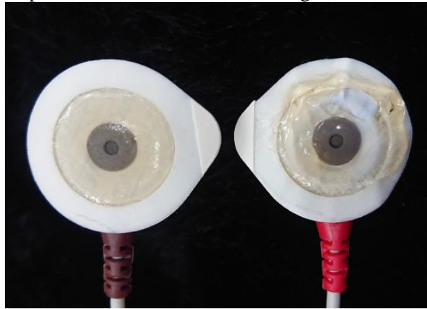
Fig. 22. Initial (left) and final (right) state of wet electrodes used during pressure variation tests.
