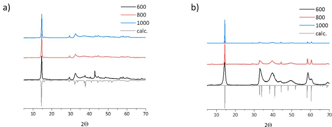
**Fig. 1.** Dependence of XRD for the ReS<sub>2</sub> (a) and MoS<sub>2</sub> (b) from the temperature T<sub>1</sub>.
