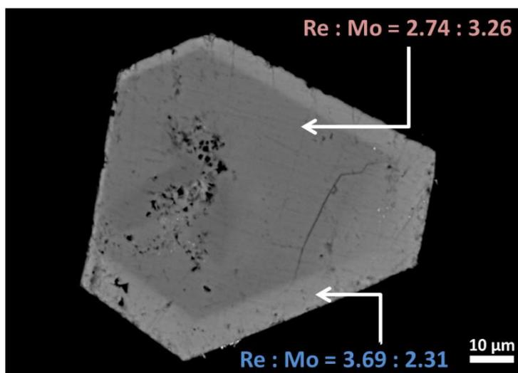
**Fig. 2.** Image of a crystal of compound **1** obtained at sintering temperature T<sub>1</sub> equal to 600°C and synthesis temperature T<sub>2</sub> equal to 750°C.
