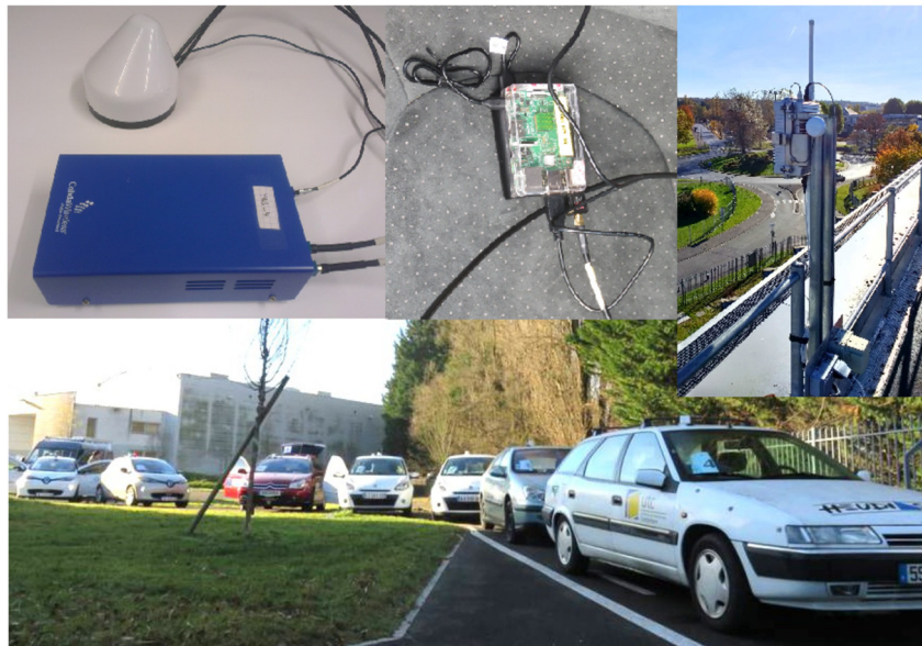
Fig. 7. Setup for the proof of concept. Top-left: IEEE 802.11p modem and roof antenna for vehicles. Top-center: Raspberry Pi running Linux, the Airplug middleware and all the applications. Top-right: IEEE 802.11p road-side-unit installed on the roof of the laboratory, close to the road. Bottom: fleet of 10 vehicles used during the road tests.
