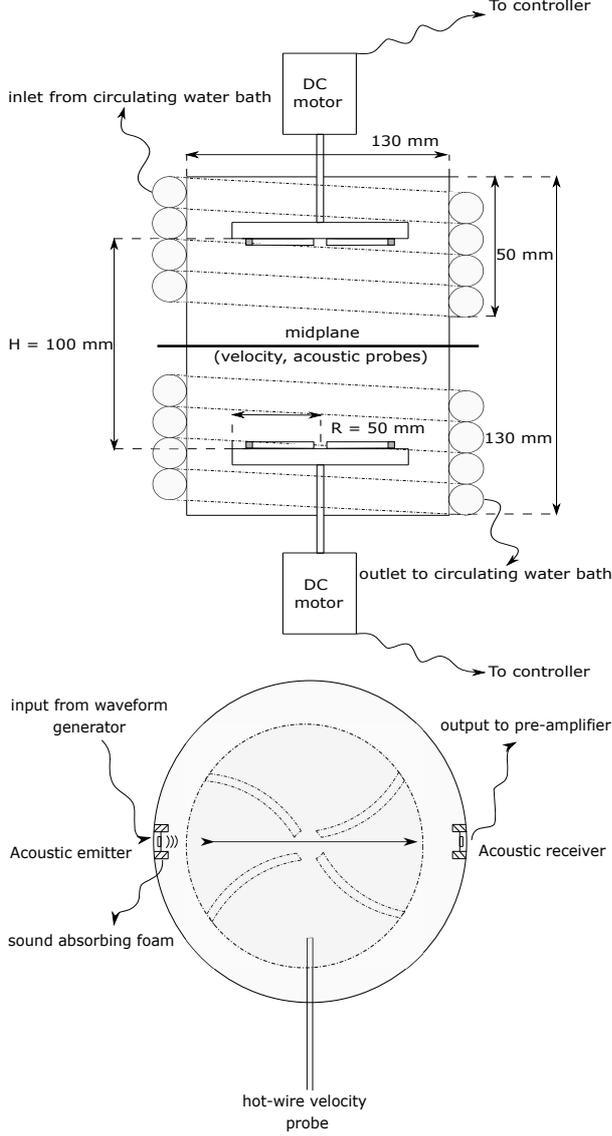
Fig. 1: Sketch of the von Kármán flow configuration driven by two counter-rotating disks. Temperature of the boundaries is maintained constant using a circulating water bath. The velocity probe and acoustic transducers are all placed in the midplane.
