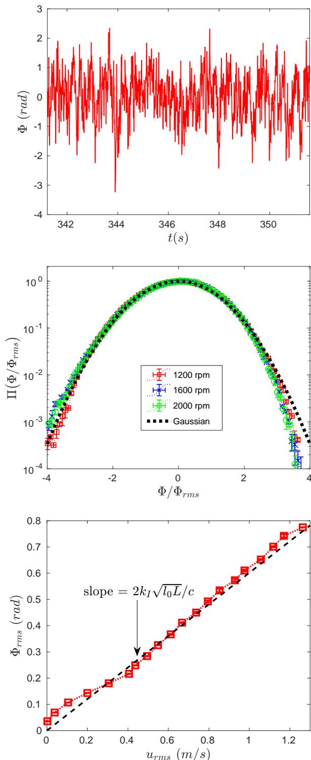
Fig. 2: (a) Time series of phase fluctuations of the incident acoustic wave for  $\Omega = 2000$  rpm. (b) PDFs of phase fluctuations normalized by their respective RMS values for  $\Omega = 1200$  rpm ( $\square$ ), 1600 rpm ( $\square$ ) and 2000 rpm ( $\square$ ). Dashed line shows the Gaussian distribution. (c) The RMS of phase fluctuations  $\Phi_{rms}$  vs the RMS of velocity fluctuations  $u_{rms}$ . Linear dependence is observed as predicted by eqn. 4.
