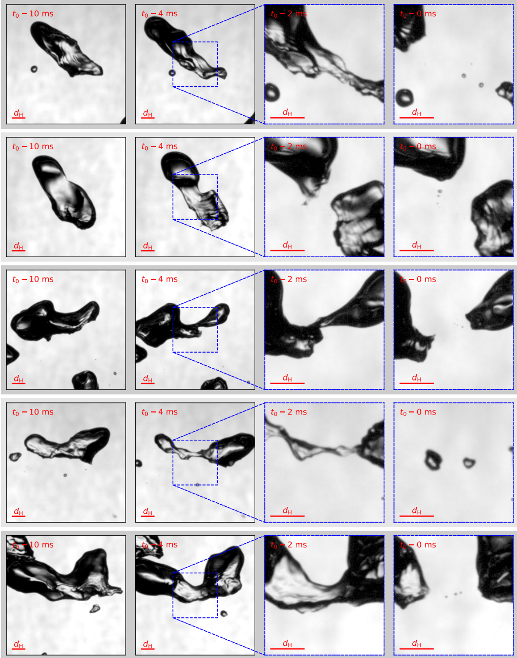
Figure 10: Five cases of sub-Hinze bubble production by the unstable collapse of a deformed ligament. Each row shows four snapshots in time, spaced 10, 4, 2, and 0 ms before the time at which the sub-Hinze bubbles are first visible. The field of view in the final two columns is given by the blue square in the second column.
