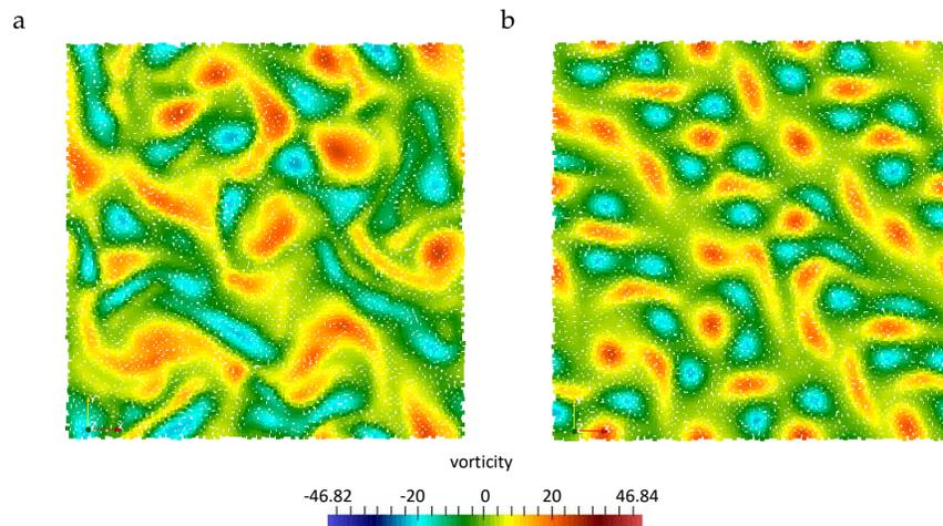
**Figure 5.** Inviscid two-dimensional Taylor–Green flow. Vorticity field for  $t = 2$ . Figure (a) shows the results using the  $\delta^+$ -SPH scheme with a constant value of  $\alpha = 0.01$ . Figure (b) shows the results obtained using the  $\delta^+$ -LES-SPH approach. Results computed using a resolution of 10,000 particles.
