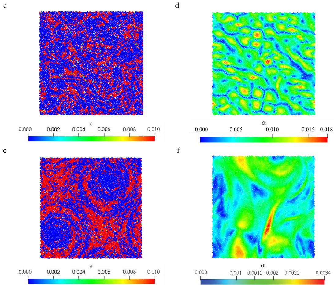
**Figure 8.** Inviscid two-dimensional Taylor–Green flow. Results for  $\epsilon$  and  $\alpha$  fields. On the left, the results obtained using the  $\delta^+$ -ADA-SPH for  $t = 0.5$  (a),  $t = 2$  (c) and  $t = 20$  (e). On the right, the results obtained using the  $\delta^+$ -LES-SPH [16] approach for  $t = 0.5$  (b),  $t = 2$  (d) and  $t = 20$  (f). Results computed using a resolution of 10,000 particles.
