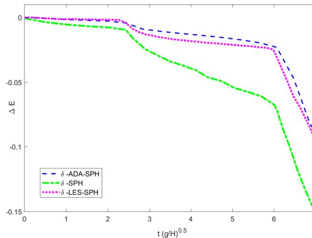
**Figure 17.** Two-dimensional dam-break flow: Time evolution of mechanical energy. The blue dashed line shows the results obtained by the present  $\delta$ -ADA-SPH scheme. The magenta dotted line presents the results obtained with the  $\delta$ -LES-SPH approach. Finally, the green dash-dot line presents the results obtained in [25] using  $\delta$ -SPH scheme. All the results are computed with  $H/\Delta x_0 = 80$ .
