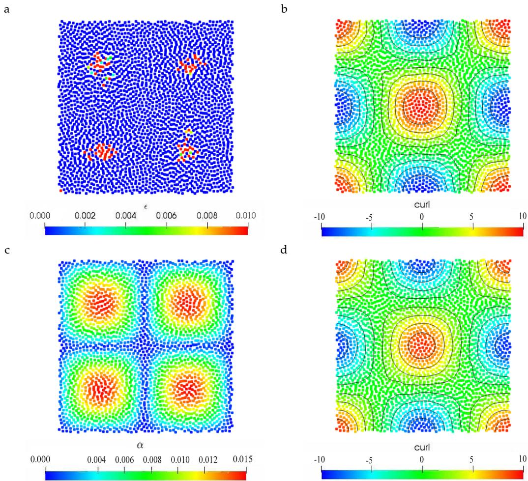
**Figure 2.** Two-dimensional Taylor–Green flow at  $Re = 1000$ . On the top, the viscosity parameter ( $\epsilon$ ) (a) and the vorticity field (b) obtained with the proposed  $\delta$ -ADA-SPH scheme. On the bottom we show the value of the  $\alpha$  parameter (c) and the vorticity field (d) using the  $\delta$ -LES-SPH. Results obtained at  $t = 3$ .
