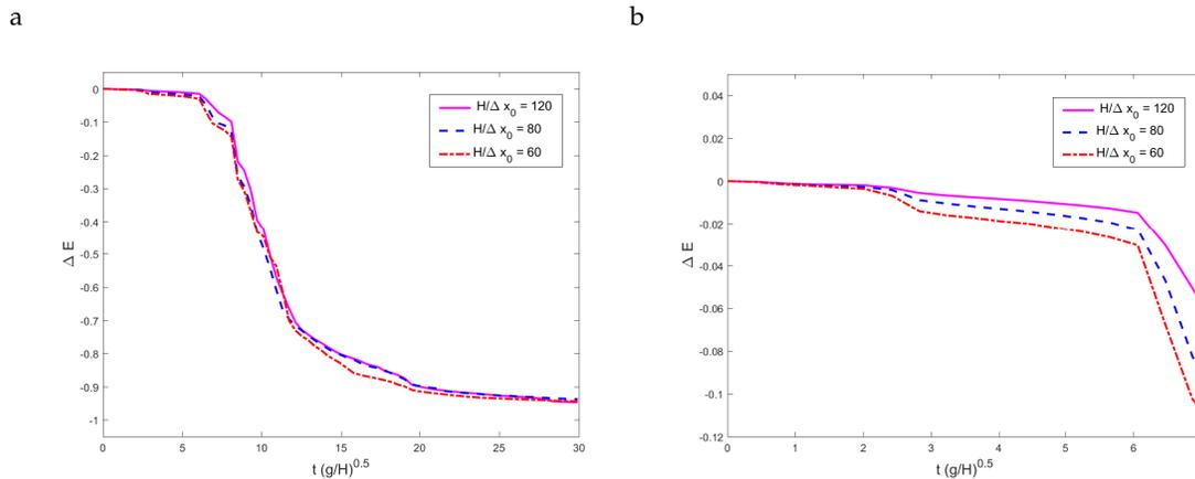
**Figure 16.** Two-dimensional dam-break flow. Figure (a) shows the time evolution of mechanical energy. Figure (b) plots the results obtained by the proposed method with different particle resolution. A zoom of the region of the curve before the first splash-up is displayed on the right.
