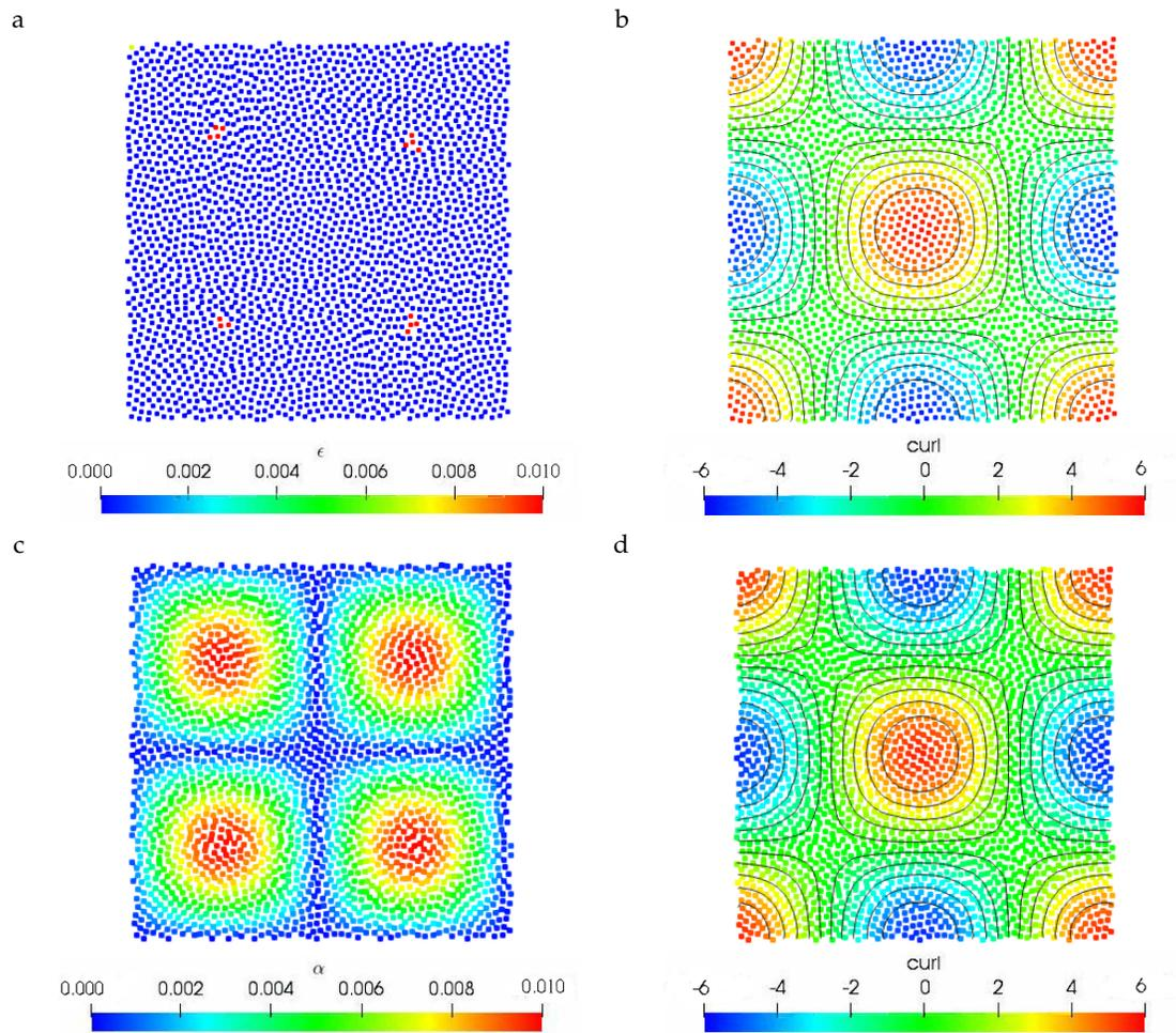
**Figure 1.** Two-dimensional Taylor–Green flow at  $Re = 100$ . On the top the viscosity parameter ( $\epsilon$ ) (a) and the vorticity field (b) obtained with the proposed  $\delta$ -ADA-SPH scheme. On the bottom we show the value of the  $\alpha$  parameter (c) and the vorticity field (d) using the  $\delta$ -LES-SPH scheme. Results obtained at  $t = 0.5$ .
