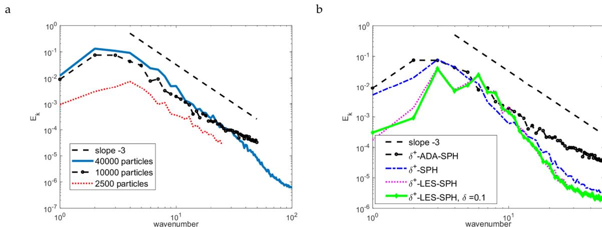
**Figure 6.** Inviscid two-dimensional Taylor–Green flow. Figure (a): Energy spectrum obtained using the proposed  $\delta^+$ -ADA-SPH method with different particle resolutions. Figure (b): comparison of the results using different  $\delta^+$ -SPH schemes using a resolution of 10,000 particles (right).
