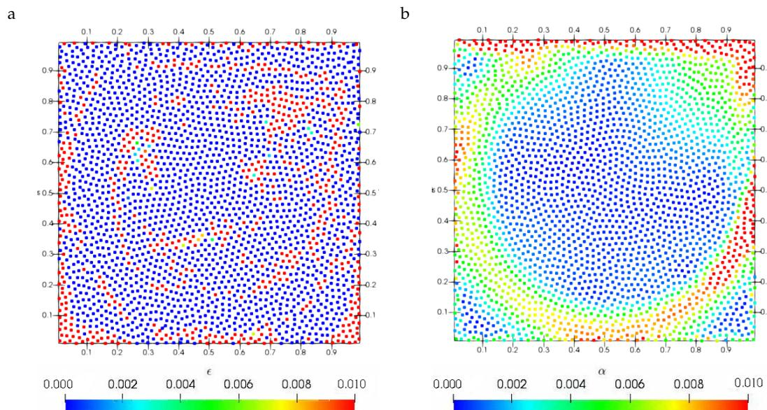
**Figure 10.** Lid-driven cavity flow: Results for  $\epsilon$  and  $\alpha$  fields for  $Re = 3200$ . Figure (a): Results obtained using the  $\delta^+$ -ADA-SPH are plotted. Figure (b): Results obtained using the  $\delta^+$ -LES-SPH [16] approach. Results computed using a resolution of  $50 \times 50$  particles.
