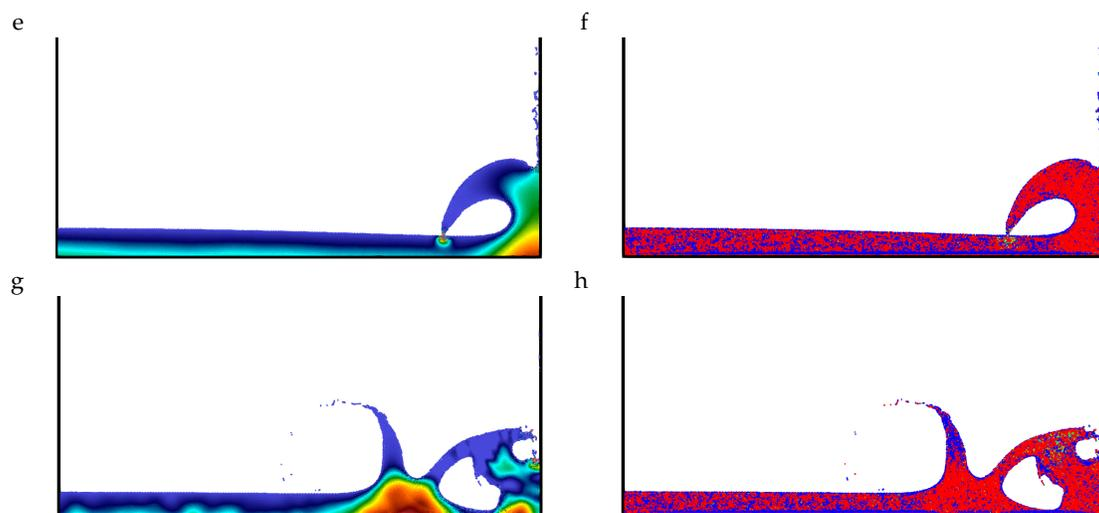
Figure 13. Two-dimensional dam-break flow: Snapshots of the computational results at different times  $t\sqrt{g/H}$  for  $H/\Delta x_0 = 120$ . On the left column the pressure field is presented,  $\epsilon$  field is placed on the right. Figures (a,b) shows the results for  $t\sqrt{g/H} = 2.35$ , (c,d) shows the results at  $t\sqrt{g/H} = 4.04$ , whereas (e,f) plots the results for  $t\sqrt{g/H} = 7.12$ . Figures (g,h) shows the results obtained at  $t\sqrt{g/H} = 7.12$ .
