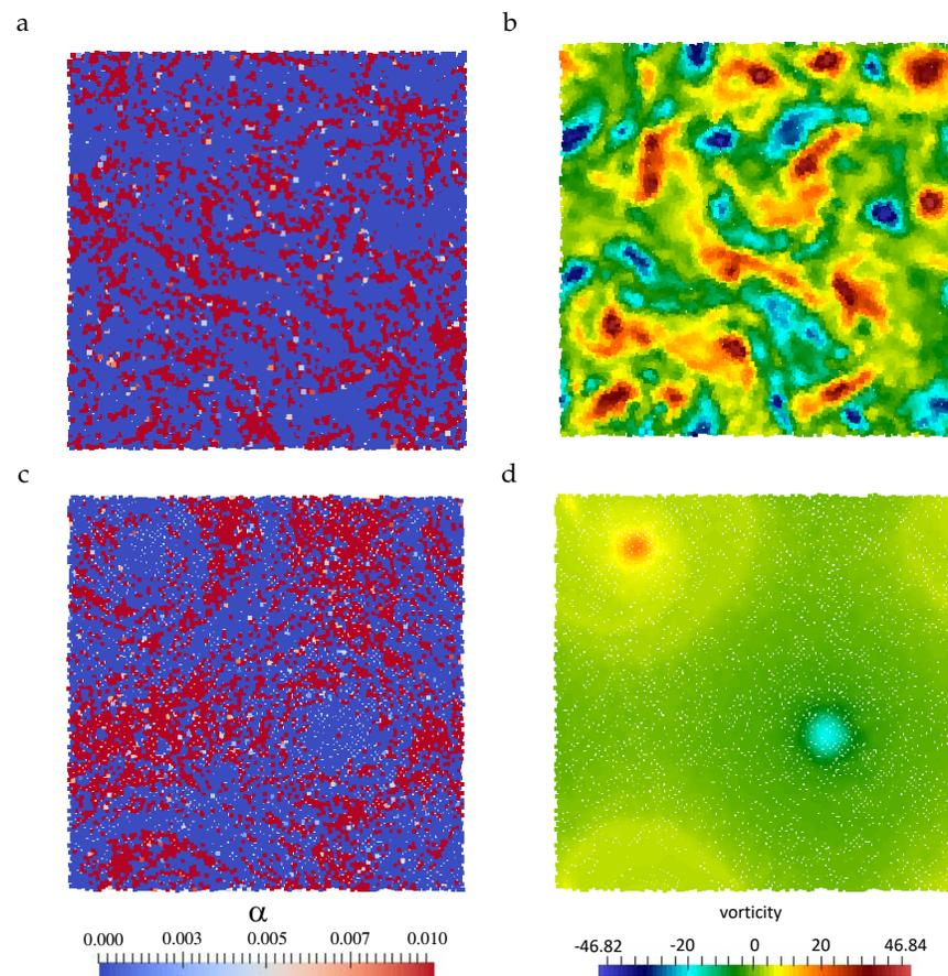
**Figure 4.** Inviscid two-dimensional Taylor–Green flow. On the left, value of  $\epsilon$  given by Equation (17). On the right, vorticity field. Figures (a,c) show the results at  $t = 2$  and figures (b,d) show the results obtained at  $t = 25$ , using a resolution of 10,000 particles.
