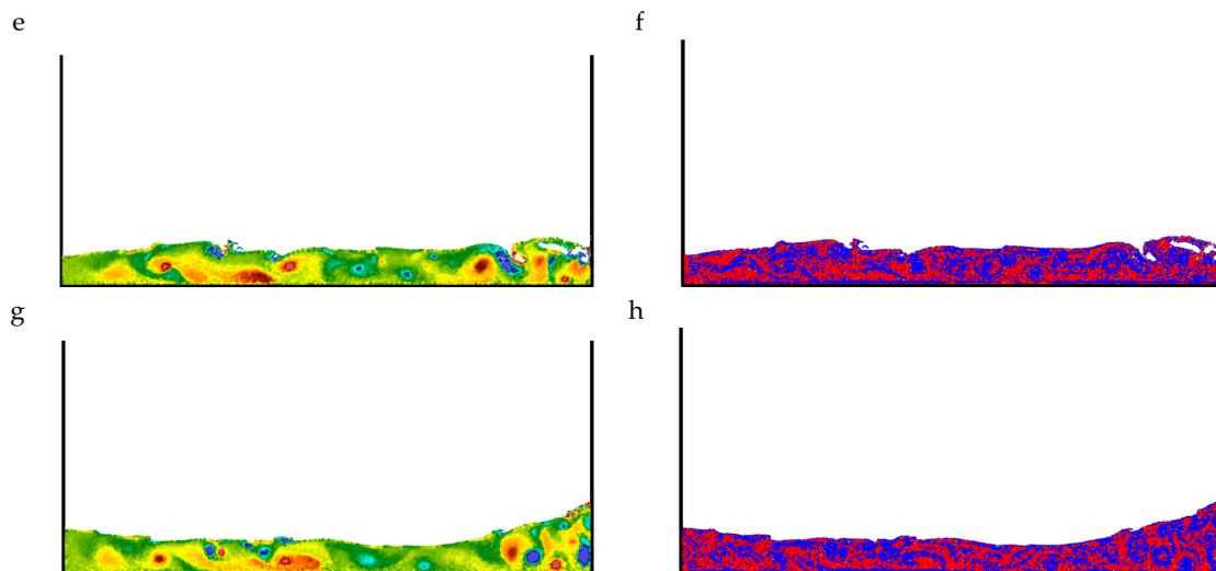
Figure 14. Two-dimensional dam-break flow: Snapshots of the computational results for different times  $t\sqrt{g/H}$  with  $H/\Delta x_0 = 120$ . On the left column the vorticity field is presented,  $\epsilon$  field is placed on the right. Figures (a,b) show the results for  $t\sqrt{g/H} = 9.54$ , (c,d) show the results at  $t\sqrt{g/H} = 13.02$ , figures (e,f) plots the results for  $t\sqrt{g/H} = 19.09$  and (g,h) shows the results obtained at  $t\sqrt{g/H} = 21.033$ .
