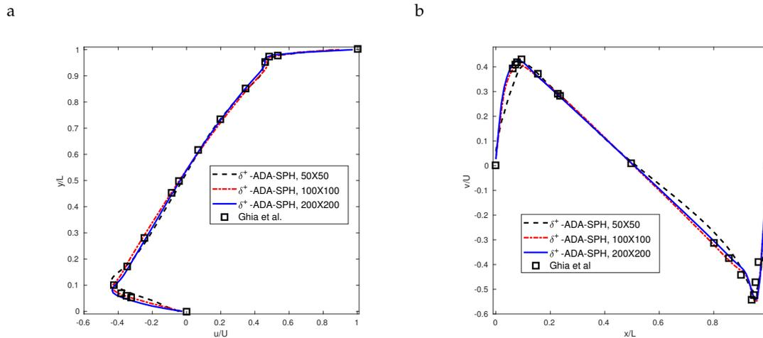
**Figure 11.** Lid-driven cavity flow: Normalized velocity profiles along vertical (a) and horizontal (b) centerlines, computed for Reynolds number  $Re = 3200$  using  $50 \times 50$ ,  $100 \times 100$  and  $200 \times 200$  particles. The solutions are compared with those of Ghia [42].
