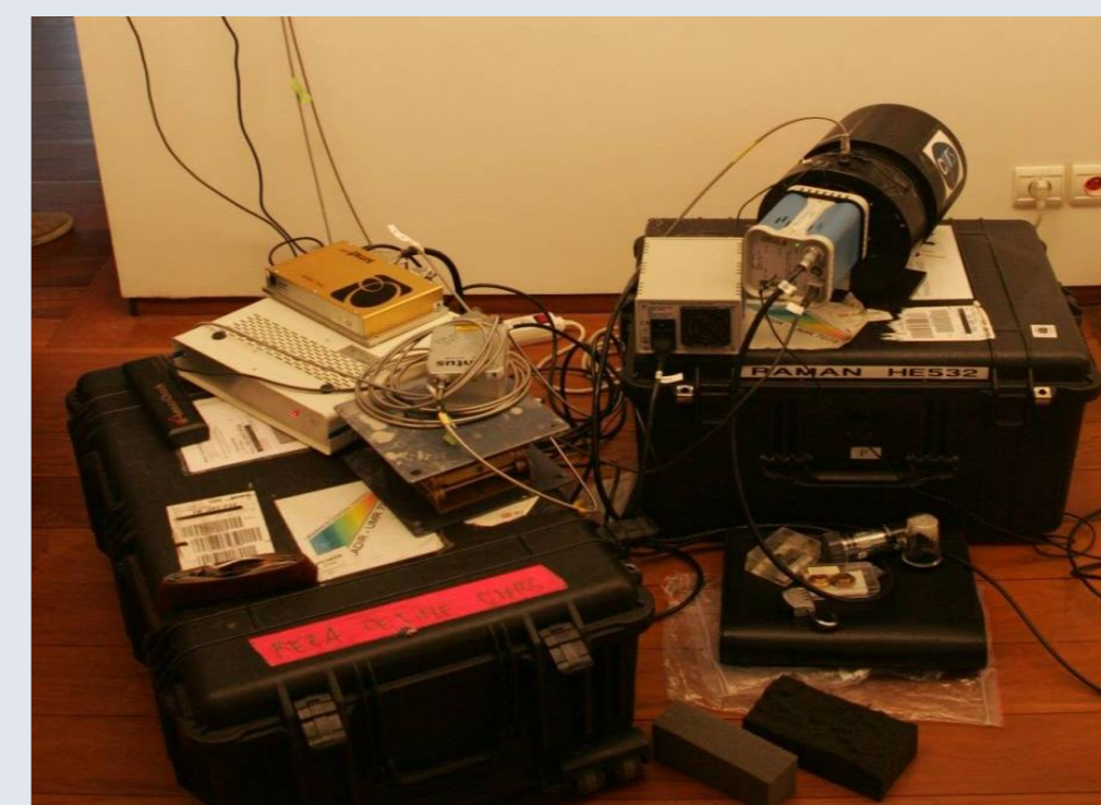
The mobile Raman spectrometer and the on-site pXRF analysis
