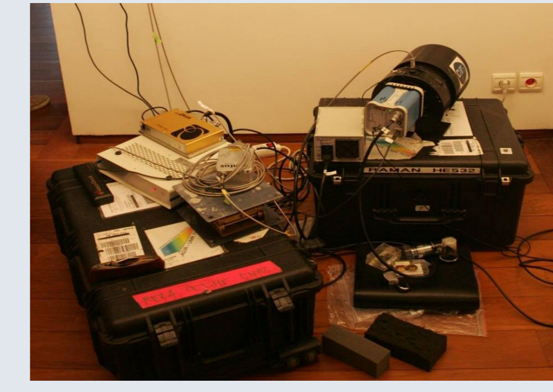
The mobile Raman spectrometer and the on-site pXRF analysis
