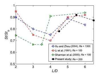
**Fig. 14.** The effect of longitudinal pitch ratio L/D on Strouhal number for two tandem cylinders in cross-flow at Re of 1300 (Xu and Zhou, 2004), 100 (Li et al., 1991; Sharman et al., 2005) and 200 (present study).
