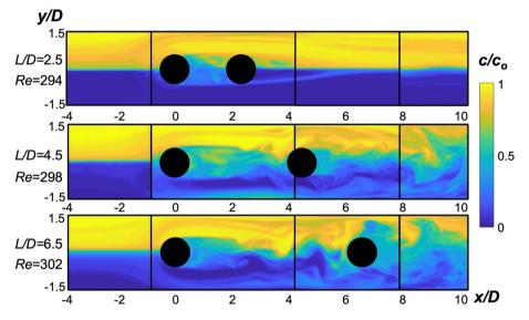
**Fig. 6.** Instantaneous normalized concentration fields for various L/D in the flow region -4 < x/D < 10, with the two mixing fluids interface set on the channel centreline, for Re  $\approx$  300. The corresponding vorticity fields are shown in Fig. 5. The fields are composites, formed by stitching together a number of overlapping segments, as discussed in Section 2.3.
