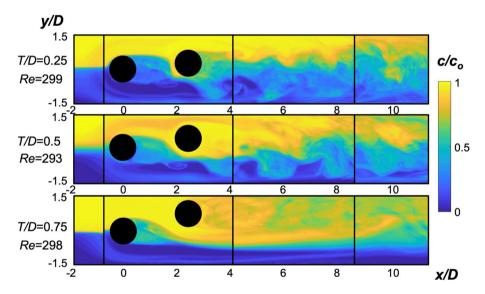
**Fig. 10.** Instantaneous normalized concentration fields for staggered cylinder pairs at various T/D in the flow region -2 < x/D < 11, with the position of inlet fluids interface set at the channel centreline. The Reynolds number  $\approx 300$  (exact values shown in labels on the left); fields correspond to vorticity maps of Fig. 9. The fields are composites, formed by stitching together a number of overlapping segments, as discussed in Section 2.3.
