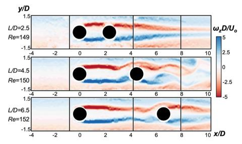
**Fig. 4.** Vorticity ( $\omega_z D/U_o$ ) contours, for microchannels with tandem cylinders (T/D = 0), for L/D = 2.5 (top row), 4.5 (middle row) and 6.5 (bottom row), for Re  $\approx$  150 (exact values shown in the figure). The vorticity fields are composites, formed by stitching together a number of overlapping segments, as discussed in Section 2.2.
