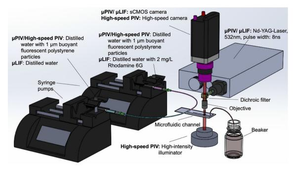
Fig. 2. Schematic of the  $\mu$ PIV and  $\mu$ LIF setup and the high-speed  $\mu$ PIV measurements.
