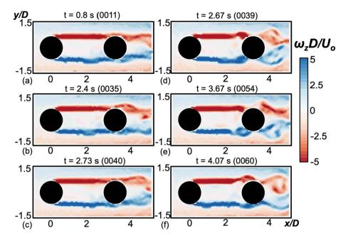
**Fig. 7.** Sample instantaneous vorticity fields for microchannels with tandem cylinders (L/D = 3.5), for Re = 299. The left columns (a-c) show instances in which the shear layers from the first cylinder reattached to the second cylinder, and the right column (d-f) show instances in which the shear layers roll up to form vortices before reaching the second cylinder.
