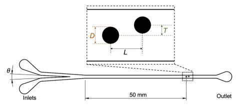
Fig.1. Schematic of a two pin microfluidic channel, showing the inlet angle ( $\theta$ ) and the definitions of the longitudinal and transverse pitch ratios (L/D and T/D).
