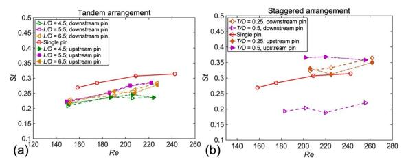
**Fig. 13.** Variation of St with Re for various values of L/D in channels with tandem cylinders (a) and T/D in channels with offset cylinders and L/D = 2.5 (b). The short-dashed and long-dashed lines represent the upstream and downstream cylinders, respectively, while the red circles denote the values found for a single cylinder under the same confinement. (For interpretation of the references to colour in this figure legend, the reader is referred to the web version of this article.)
