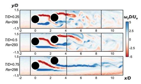
**Fig. 9.** Vorticity ontours  $\omega_z D/U_o$  for microchannels with cylinders in staggered (L/D = 2.5) and T/D ranging from 0.25 to 0.75. The Reynolds number  $\approx$  300 (exact values shown in labels on the left). The fields are composites, formed by stitching together a number of overlapping segments, as discussed in Section 2.2.
