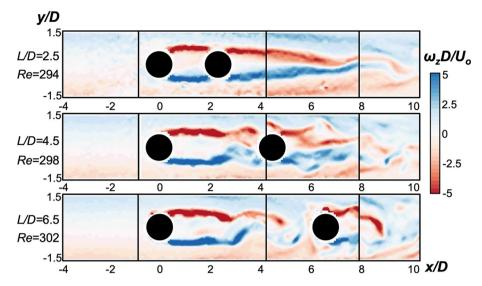
**Fig. 5.** Vorticity ( $\omega_z D/U_o$ ) contours for microchannels with tandem cylinders (T/D = 0), for L/D = 2.5 (top row), 4.5 (middle row) and 6.5 (bottom row), for Re  $\approx$  300 (exact values shown in the figure). The vorticity fields are composites, formed by stitching together a number of overlapping segments, as discussed in Section 2.2.
