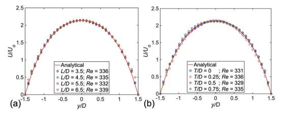
Fig. 3. Comparisons between experimental velocity profiles for microchannels with (a) T/D fixed at 0 and various L/D and (b) L/D fixed at 2.5 and various T/D as well as analytical (solid line) velocity profiles (x/D = -5, z/D = 0) for Re around 335 (exact values shown in the figure).
