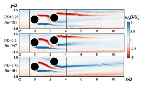
**Fig. 8.** Vorticity contours  $\omega_z D/U_o$  for microchannels with cylinders in staggered (L/D = 2.5) and T/D ranging from 0.25 to 0.75. The Reynolds number  $\approx$  150 (exact values shown in labels on the left). The fields are composites, formed by stitching together a number of overlapping segments, as discussed in Section 2.2.
