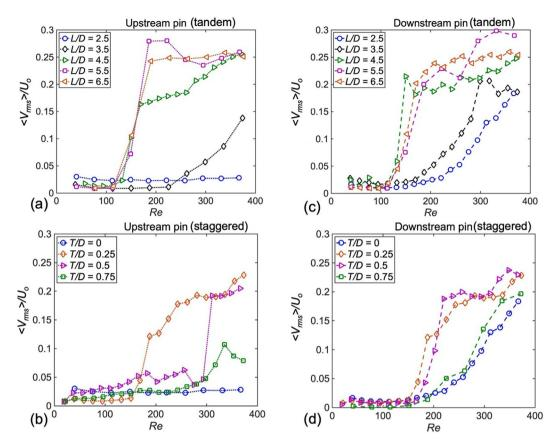
**Fig. 11.** Variation of the mean  $< V_{rms} > /U_o$  calculated in the wake of the upstream (a) and downstream (b) tandem cylinders, and is the wake of the upstream (c) and downstream (d) staggered cylinders, for which L/D = 2.5. The regions over which the averages were calculated are discussed in the text.
