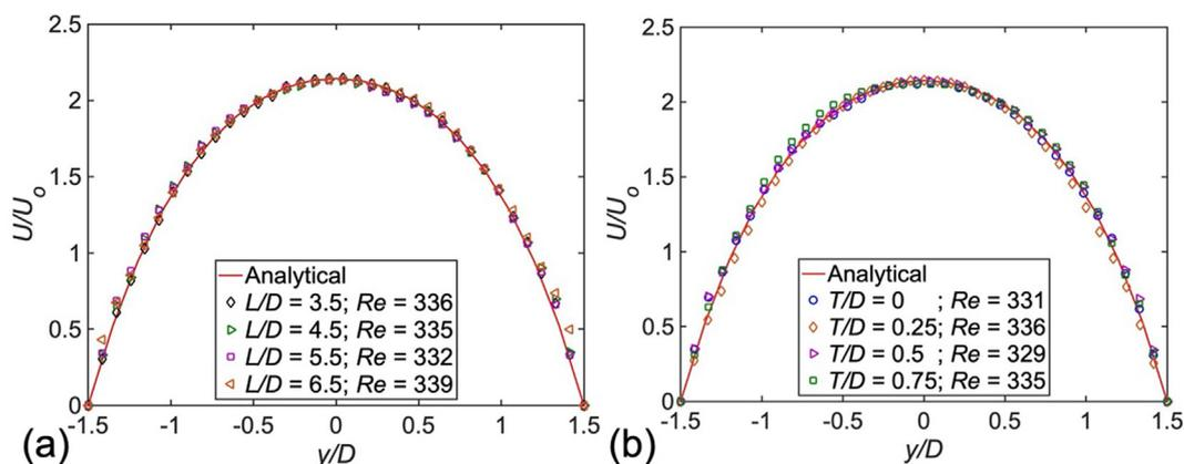
**Fig. 3.** Comparisons between experimental velocity profiles for microchannels with (a)  $T/D$  fixed at 0 and various  $L/D$  and (b)  $L/D$  fixed at 2.5 and various  $T/D$  as well as analytical (solid line) velocity profiles ( $x/D = -5$ ,  $z/D = 0$ ) for  $Re$  around 335 (exact values shown in the figure).
