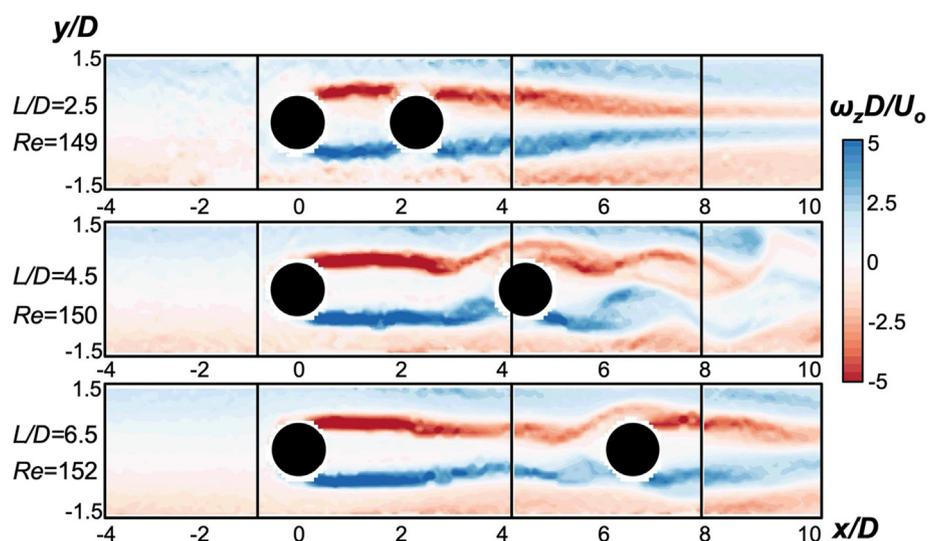
**Fig. 4.** Vorticity ( $\omega_z D/U_0$ ) contours, for microchannels with tandem cylinders ( $T/D = 0$ ), for  $L/D = 2.5$  (top row), 4.5 (middle row) and 6.5 (bottom row), for  $Re \approx 150$  (exact values shown in the figure). The vorticity fields are composites, formed by stitching together a number of overlapping segments, as discussed in Section 2.2.
