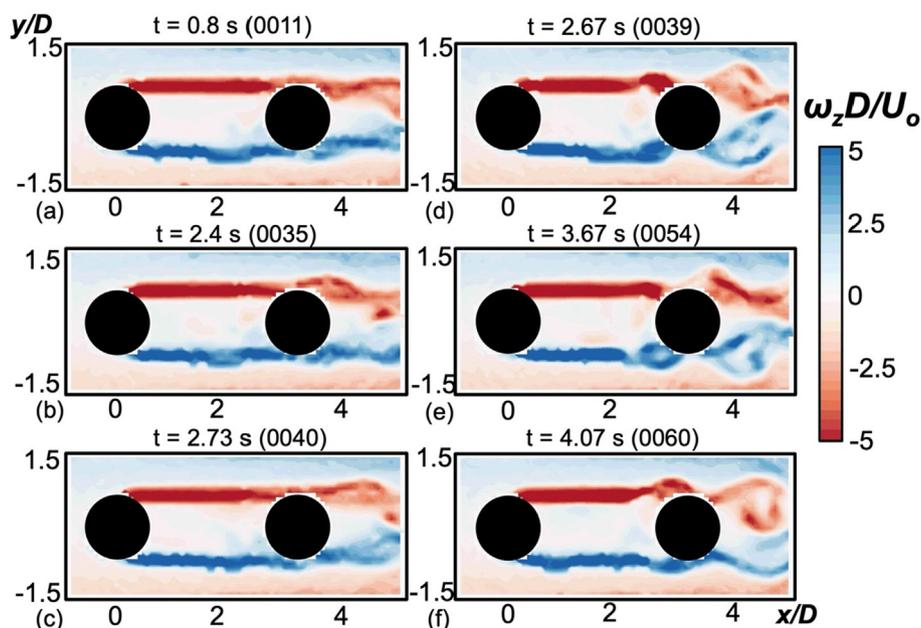
**Fig. 7.** Sample instantaneous vorticity fields for microchannels with tandem cylinders ( $L/D = 3.5$ ), for  $Re = 299$ . The left columns (a-c) show instances in which the shear layers from the first cylinder reattached to the second cylinder, and the right column (d-f) show instances in which the shear layers roll up to form vortices before reaching the second cylinder.
