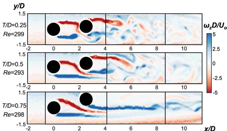
**Fig. 9.** Vorticity contours  $\omega_z D/U_0$  for microchannels with cylinders in staggered ( $L/D = 2.5$ ) and  $T/D$  ranging from 0.25 to 0.75. The Reynolds number  $\approx 300$  (exact values shown in labels on the left). The fields are composites, formed by stitching together a number of overlapping segments, as discussed in Section 2.2.
