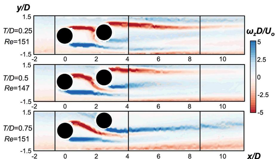
**Fig. 8.** Vorticity contours  $\omega_z D/U_0$  for microchannels with cylinders in staggered ( $L/D = 2.5$ ) and  $T/D$  ranging from 0.25 to 0.75. The Reynolds number  $\approx 150$  (exact values shown in labels on the left). The fields are composites, formed by stitching together a number of overlapping segments, as discussed in Section 2.2.
