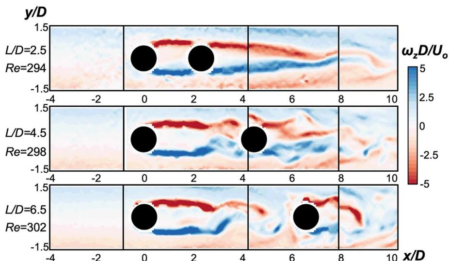
**Fig. 5.** Vorticity ( $\omega_z D/U_0$ ) contours for microchannels with tandem cylinders ( $T/D = 0$ ), for  $L/D = 2.5$  (top row),  $4.5$  (middle row) and  $6.5$  (bottom row), for  $Re \approx 300$  (exact values shown in the figure). The vorticity fields are composites, formed by stitching together a number of overlapping segments, as discussed in Section 2.2.
