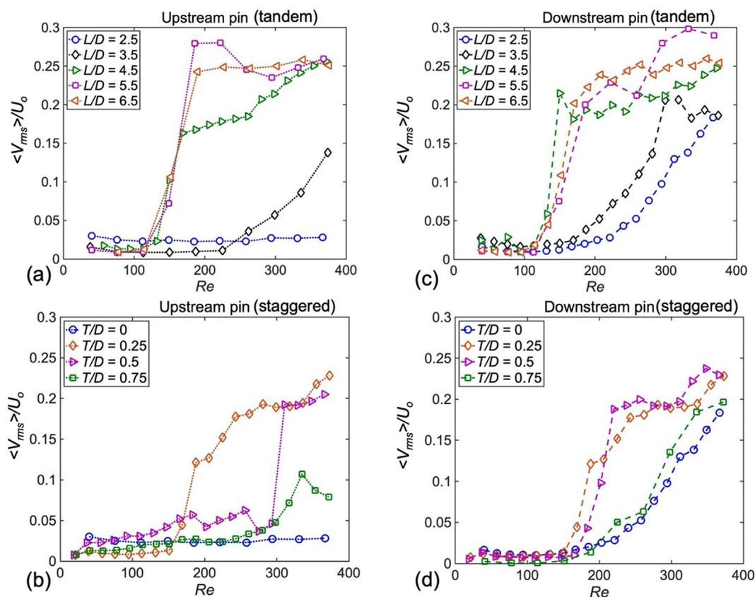
**Fig. 11.** Variation of the mean  $\langle V_{rms} \rangle / U_0$  calculated in the wake of the upstream (a) and downstream (b) tandem cylinders, and is the wake of the upstream (c) and downstream (d) staggered cylinders, for which  $L/D = 2.5$ . The regions over which the averages were calculated are discussed in the text.
