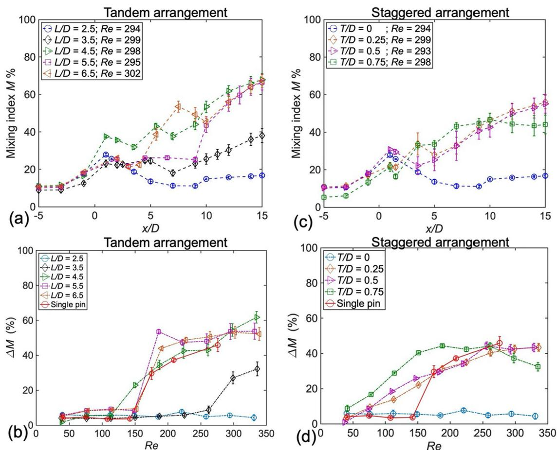
**Fig. 15.** The variation of the mixing index along the channel ( $x/D = -5$  to  $15$ ) for channels with tandem cylinders (a) and staggered cylinders (c) at  $Re \approx 300$ , and the percentage increase in  $M$  over the measurement region as a function of  $Re$  for tandem (b) and staggered (d) cylinders. Note that some of the symbols are larger than the error bars, which are computed as the standard deviation over the 100 fields.
