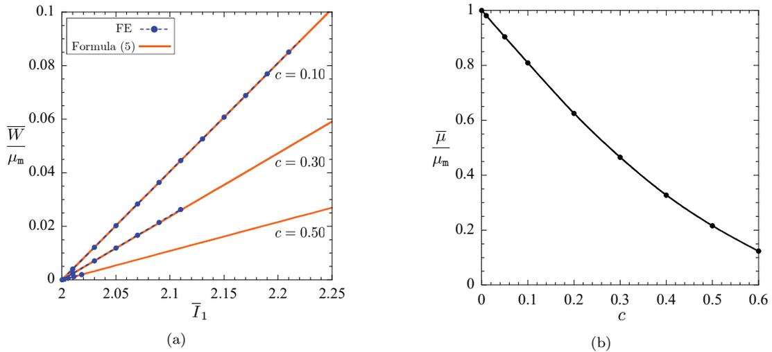
Fig. 3: (a) FE results for the effective stored-energy function (3) for Neo-Hookean composites made of a Neo-Hookean matrix filled with circular liquid ( $\mu_p = \mu_m/100$ ) particles at several concentrations  $c$  as functions of the deformation measure  $\bar{I}_1 = \bar{\mathbf{F}} \cdot \bar{\mathbf{F}}$ . (b) The corresponding effective shear modulus (6) in the conjectured formula (5), which is also plotted in part (a) for direct comparison with the FE results, as a function of  $c$ .
