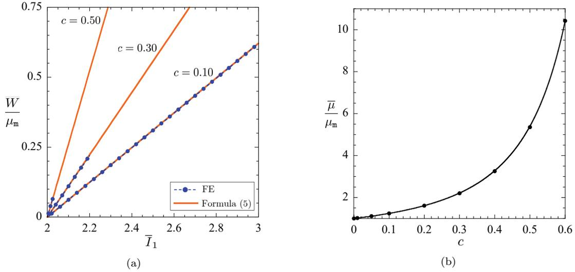
Fig. 2: (a) FE results for the effective stored-energy function (3) for Neo-Hookean composites made of a Neo-Hookean matrix filled with circular rigid ( $\mu_p = +\infty$ ) particles at several concentrations  $c$  as functions of the deformation measure  $\bar{I}_1 = \bar{\mathbf{F}} \cdot \bar{\mathbf{F}}$ . (b) The corresponding effective shear modulus (6) in the conjectured formula (5), which is also plotted in part (a) for direct comparison with the FE results, as a function of  $c$ .
