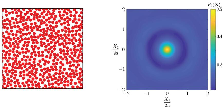
Fig. 1: Representative unit cell  $Y_0$  containing a random distribution of  $N = 480$  monodisperse circular particles at concentration  $c = 0.50$  and the contour plot of its two-point correlation function  $P_2(\mathbf{X})$  near the origin  $\mathbf{X} = \mathbf{0}$  as a function of the coordinates  $X_1$  and  $X_2$  normalized by the diameter  $2a$  of the particles.
