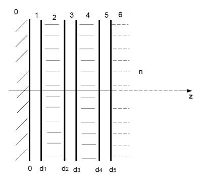
FIG. 1: A N layer cavity. For the dielectric case in the 0, 2, 4, ..., and all even-numbered regions there is a dielectric and in the 1, 3, 5, ..., and all odd-numbered regions there is vacuum.  $d_i$  is the thickness of the *i*-th slab. In the case of plasma-sheet there is vacuum everywhere and the layer are simple interfaces (of zero thickness) at  $z = d_1, d_2, ...$
