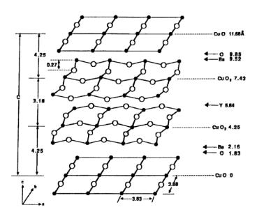
FIG. 5: Typical layered structure of  $YBa_2Cu_3O_7$  [20].
