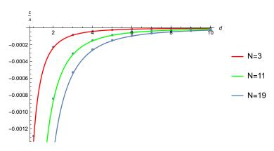
FIG. 3: A comparison between exact numerical values of the Casimir energy (dots) and the approximated formula, Eq. (7) (lines), with d expressed in nm and E/A in  $J/m^2$ .
