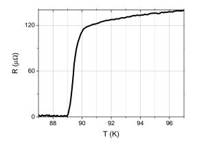
FIG. 6: The transition of the sample of YBCO we are using.
