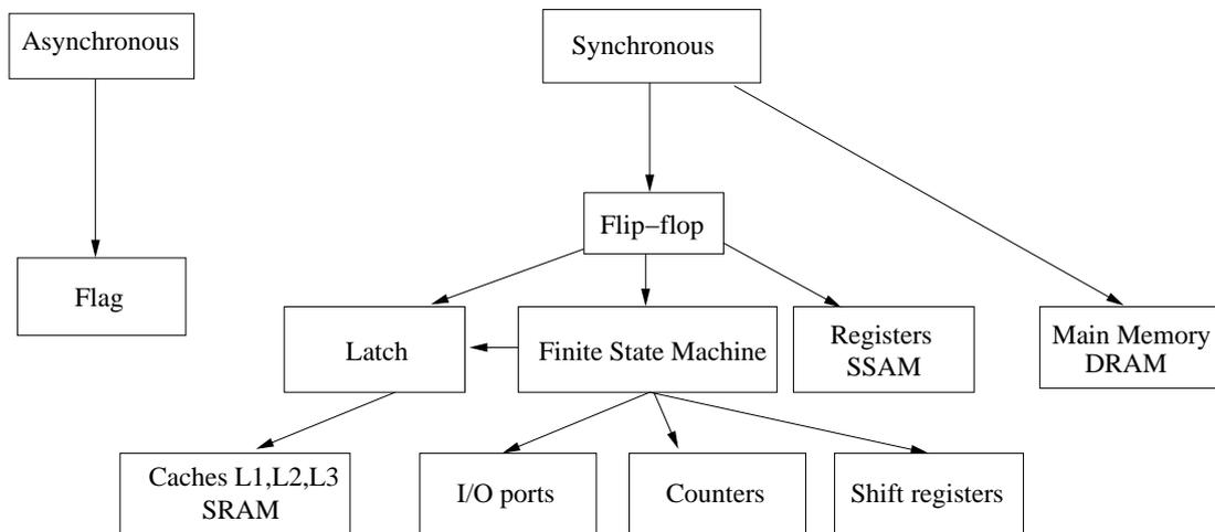
**Fig.2:** Sequential logic family tree. SRAM is Static Random Access Memory whereas SSAM is Static Sequential Access Memory. DRAM is Dynamic RAM (originating from the capacitor refreshment process). Memory types are Static (logic based) or Dynamic (Transistor and Capacitor based).
