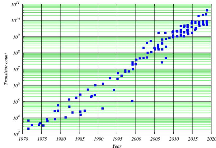
**Fig.1:** Moore's law illustrated with transistor count in a CPU chip from the beginning of circuit integration circa 1970 to present times. The chips originate from Intel, Apple, AMD, Motorola, ARM and SUN Microsystems. Data gathered by Hannah Ritchie and Max Roser under CC-BY Licence.
