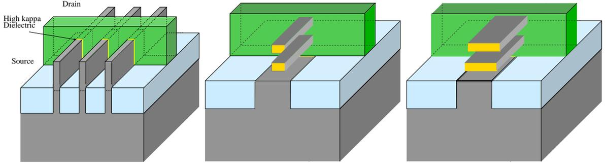
**Fig.7:** (Color on line) Architecture of the 3D FinFET, GAAFET (Gate-All-Around) and MBCFET (Muti-Bridge Channel) devices. Three fins linking source to drain are displayed in the FinFET, whereas two nanowires are shown in the GAAFET and two nanosheets (ribbons) are used in the MBCFET. Adapted from Tech-Brief [9].
