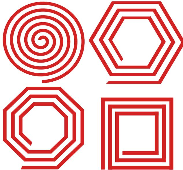
**Fig.5:** Flat inductors [7] with circular, hexagonal, octagonal and square shapes are used to increase  $Q$  when lying over an insulator substrate or simply suspended over it in order to decrease losses.
